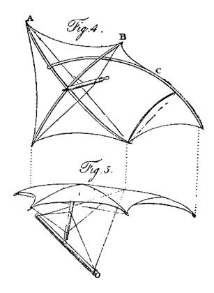
This fabrick contained 54 square feet, and weighed only eleven pounds. Although both these wings together did not compose more than half the surface necessary for the support of a man in the air, yet during their waft they lifted the weight of nine stone. The hinder edge, as is evident from the construction, being capable of giving way to the resistance of the air, any degree of obliquity, for the purpose of a propelling power, may be used.
