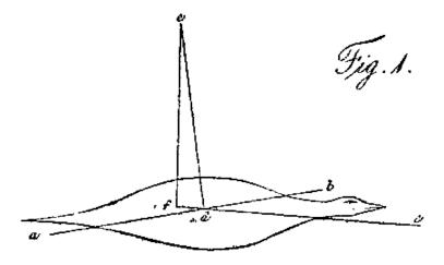
Let *a b* be a section of the plane of both wings opposing the horizontal current of the air (created by its own motion) which may be represented by the line *c d*, and is the measure of the velocity of the bird. The angle *b d c* can be increased at the will of the bird, and to preserve a perfectly horizontal path, without the wing being
