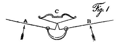
Another principle, that may be applied to obviate this leverage of a wing, is that of using such a construction as will make the supporting power of the air counterbalance itself. It has been before observed, that only about one third of the wing in birds is applied in producing the propelling power; the remainder, not having velocity sufficient for this purpose, is employed in giving support, both in the beat and return of the wing.
