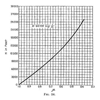
In practice, however, it happens that the temperature of the air also decreases as one rises above the ground. Then at a given height H, the density  $\mu$  with respect to the ground level, is greater than the value given by the above formula. In the following discussion, which is primarily qualitative in nature, we will not take into account this decrease in temperature, in order not to complicate the treatment of the subject.
