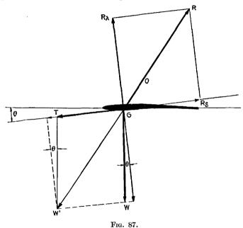
force will appear, other than the weight W and air reaction R, namely, the propeller thrust, T.
