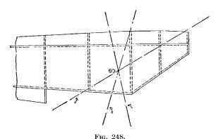
balancing the machine on the wheels; v''' will then be the vertical which passes through the axis of the wheels (Fig. 247). The three lines v', v'' and v''' must meet in a point (Fig. 248).
