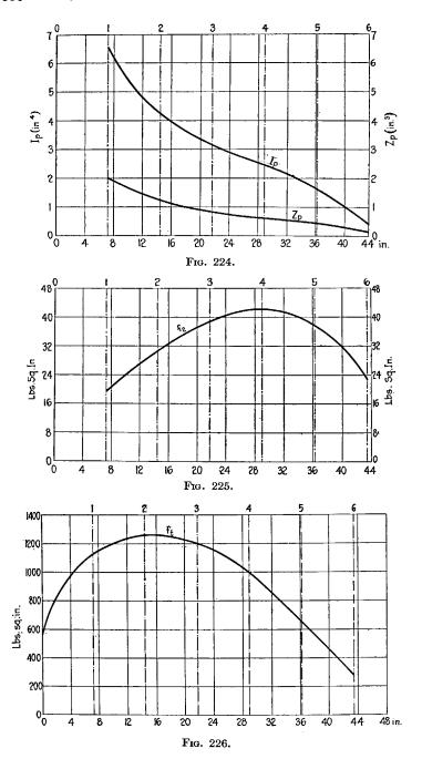
It is now necessary to determine the polar moments  $I_p$  of the various sections; to this effect it suffices to determine the ellipse of inertia of the various sections by the usual methods of graphic analysis; then calling  $I_x$  and  $I_y$  the moments of inertia with respect to the principal axis of inertia, we will have
