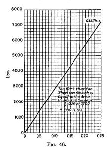
cent.; the work that it can absorb is equal as shown in the diagram to 1800 ft.-lb. As this gives a total of 2700 ft.-lb.,
