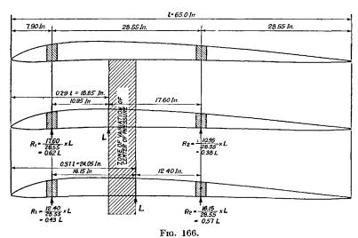
applied in a directly opposite direction to the air reaction, decreases the value of the reaction. In our case the figured weight of the wing truss is 276 lb.; thus the weight per linear inch to be subtracted from the preceding values will be 0.45 lb. per linear inch.
