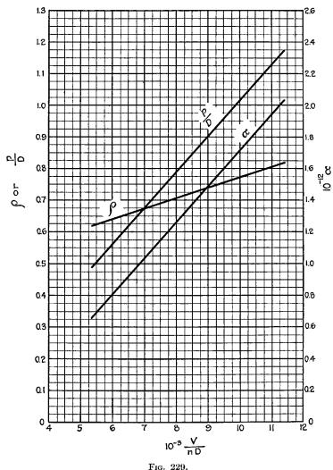
propellers of the best known type to-day, with the indication of the values  $\frac{V}{nD}$ ,  $\alpha = \frac{P}{n^3D^5}$  and  $\frac{p}{D}$  corresponding to the value of maximum efficiency, adopting as units, how-
