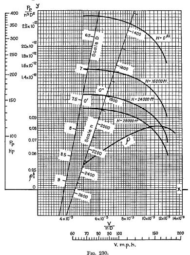
By using these diagrams those of Fig. 232 have been drawn from which it is seen that the maximum velocity at sea level is only 150 m.p.h. with a corresponding useful power of 225 H.P. This depends upon the fact that a pro-
