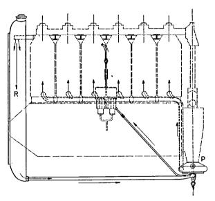
Fig. 57.—Water-cooling system.
