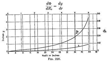
that is, that the resultant of  $d\Phi$  and  $dR_t$  be tangent to the neutral curve of the propeller blade. Under these conditions, supposing that this be true for every element  $A \times dr$  of the propeller, all the various sections will be stressed only to tension.
