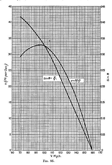
series of speeds, varying from a minimum value, which depends essentially upon the characteristics of the airplane, to a maximum value which depends not only upon the airplane, but also upon the engine and propeller.
