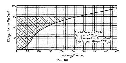
wrapping. The work can be easily calculated by measuring the shaded areas in Figs. 153 and 154. Naturally to do this it is necessary to translate the per cent. scale of elongation into inches, which is easy when the weight per yard is known.
