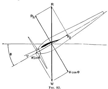
the airplane is well balanced, it will follow a sloping line of path  $\theta$  (Fig. 82), which will make a well-determined angle of incidence i, with the wing; in fact, if this angle should vary, some restoring couples (see Chapter II), tending to keep the machine at incidence i, would be produced.
