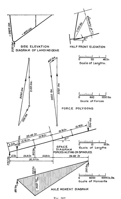
because with a great transversal load the wheel would break. In Fig. 209 the sections of the various members have been given, the results of the analysis having been CASE 4.
