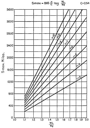
reduce the specific consumption to half, the radius of action would be doubled.
