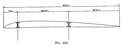
different values as there are angles of incidence. The maximum value, which is assumed in computations, is, usually, D = 0.25. Thus it will be sufficient to study the distribution of L, because, when this is known the horizontal stresses can immediately be calculated.
