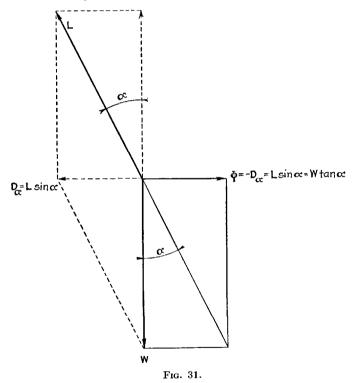
this cannot be actually done in practice since there is a possibility of the machine banking while turning. Now, when the airplane "banks," the forces L and W will admit a lateral resultant  $D_{\alpha}$  which tends to deviate laterally the line of flight. A centrifugal force  $\Phi$  is thereby developed, tending to balance the force  $D_{\alpha}$  and equilibrium will obtain when  $\Phi = D_{\alpha}$  (Fig. 31); that is, when
