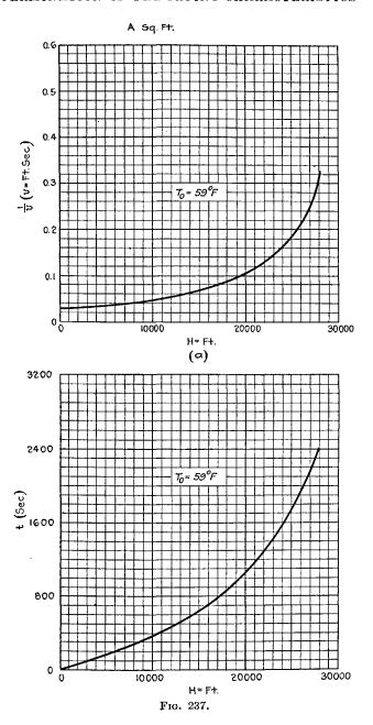
9 ft. This propeller is the one for which the static analysis was given in the preceding chapter. For such a propeller the logarithmic diagrams of  $\rho P_2$ , the diagram v = f(H) and those of  $\frac{l}{v} = f(H)$  and t = f(H) have been plotted in figures 235, 236 and 237ab respectively.
