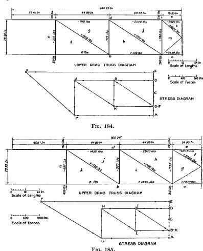
which is doubly compressed. In order to take the stress from it, at least partially, it is practical to adopt drag cables which anchor the wings horizontally. Usually these drag cables anchor the upper wings only. Sometimes also the lower ones.
