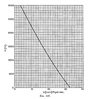
giving the time spent by the airplane in reaching a certain height H. To construct this diagram it is necessary first of all to draw the diagram of the equation
