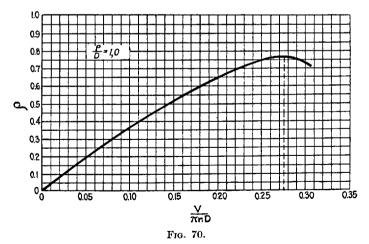
On the contrary, it is of maximum interest to examine equation (3), which gives the efficiency of the propeller. Let us consider all geometrically similar propellers of the same family, having diameter D and pitch p, so that  $\frac{p}{D}$
