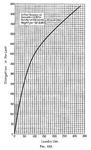
work that the elastic can absorb. The diagrams of Figs. 153 and 154 show this clearly.
