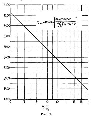
We wish to show now, how, with sufficient practical approximation, it is possible to reduce the formula which gives  $H_{\text{max}}$ , to become solely a function of W,  $P_2$  and A; that is, of the three elements which are always known in an airplane. In fact the values of  $\rho$  and  $\lambda_{\text{max}}$  for the greatest
