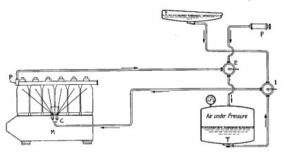
Fig. 55.—Gasoline pressure feed system.
