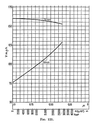
the motive power is not effected by the variation of the air density but keeps constant at the various heights. We shall see immediately that in this case the propeller will greatly increase the number of revolutions; it is then necessary to extend the characteristics of the engine above 2200 revolutions per minute.
