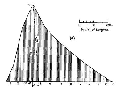
MOMENT DIAGRAM FOR ELEVATOR LOADS AND TEN TIMES THE FUSELAGE WEIGHTS
