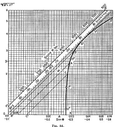
ficient in order that a system of values of W, V and  $-\sin\theta$  be realizable with the given airplane, is evidently that the three corresponding segments, summed geometrically starting from the origin, end on the diagram.
