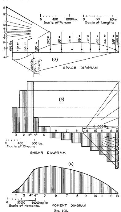
(c) For maneuvering the rudder the same applies as for the elevator. The same diagrams of Fig. 198 may also be used for this case.
