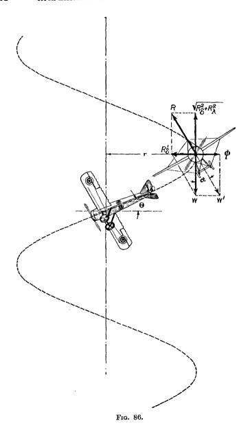
force is provoked solely by the inclination of the airplane, that is, when the angle of drift is zero, we say the spiral descent is correct, the machine then doesn't turn flat; as in practice this is the normal case, we shall study only this case. We developed the discussion for this case as if the weight were increased from W to W' where
