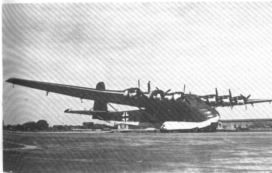
Messerschmitt Me 323 aeroplane. Although rated for 200 passengers as a glider, on at least one flight, the Me 323 transported 240 men (eighty in the wings, 160 in the fuselage) to Sicily from North Africa despite the added weight of the six engines
