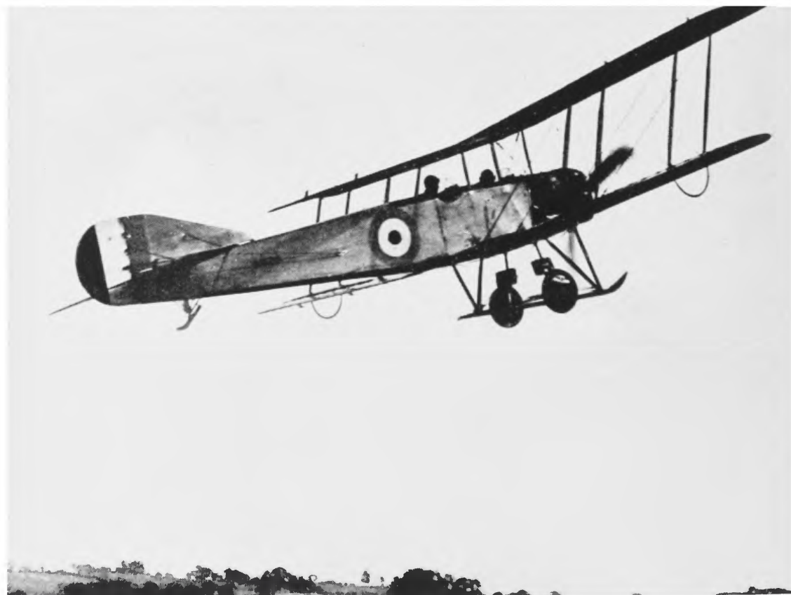
9 An Avro 504B, designed by Sir A. Verdon-Roe, with an 80 h.p. Gnome engine
