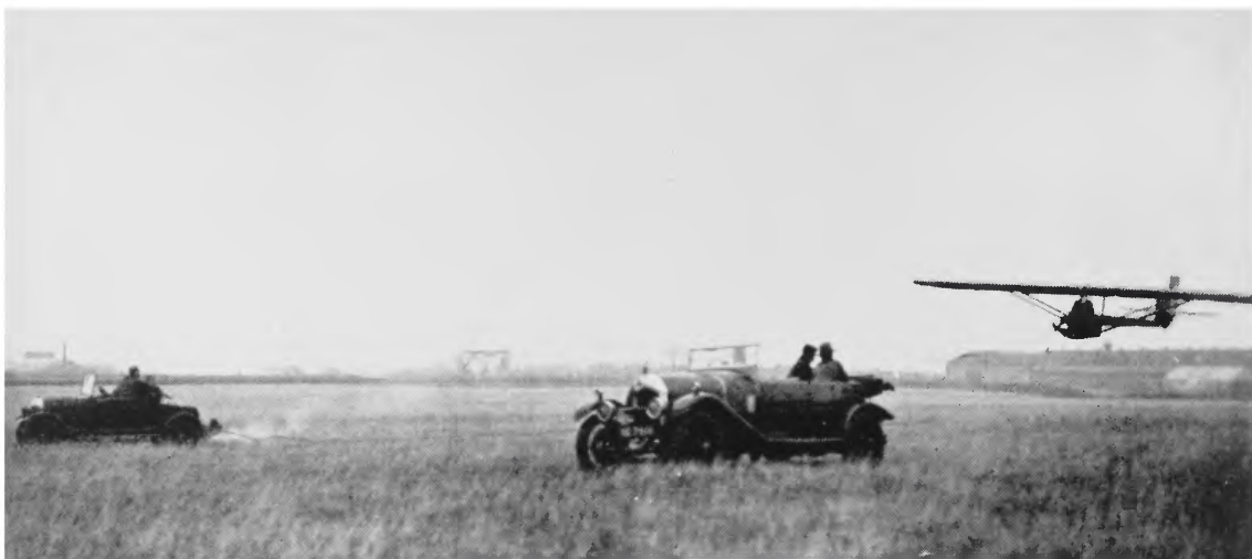
49 Experimenting with launching a glider by a tow rope stretched between two motor-cars at East Cowes, 1930
