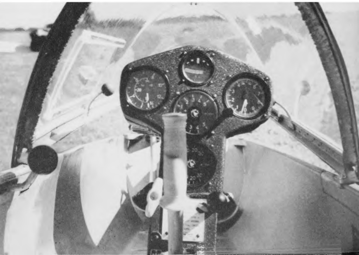
Below: Instrument panel of a modern glider.
