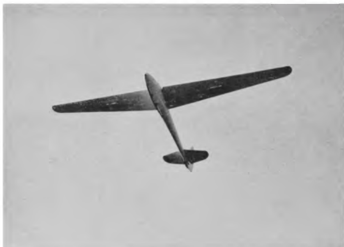
PLATE 10. The Weihe, a German high-efficiency plane flown by the author. It is notable for its natural stability and great powers of penetration.
