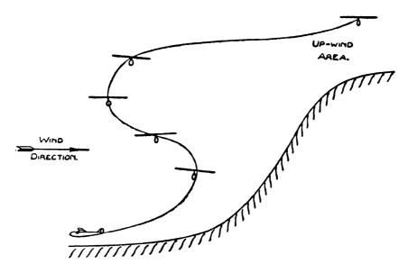
Fig. 23.—Landing after Soaring Flight.
