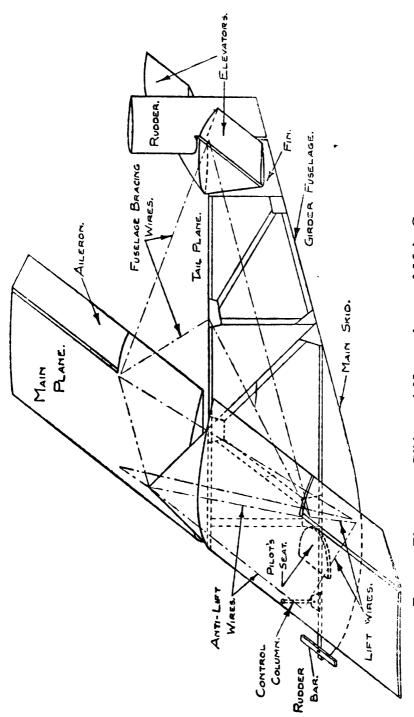
Fig. 1.—Elementary Glider and Nomenclature of Main Components.
