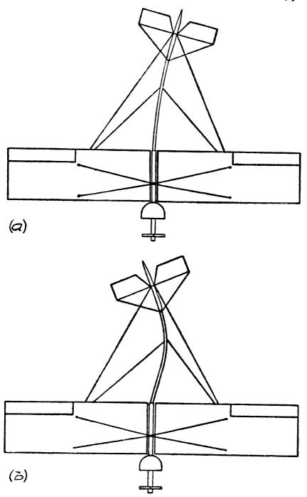
Fig. 16.—Rigging Faults.
