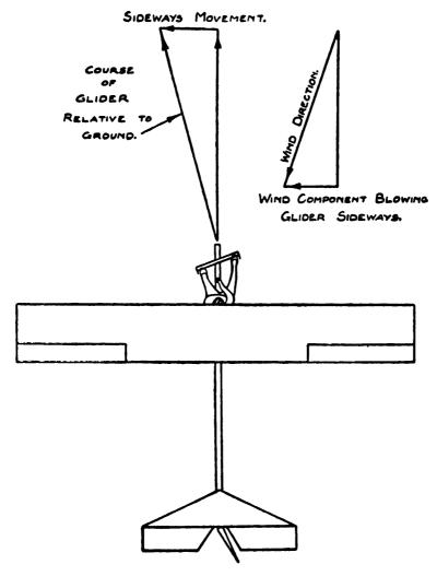
Fig. 19.—Correction of Drift.
