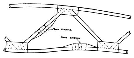
Fig. 41.—Repairs to Rib.
