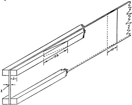
Fig. 31.—Splices in Spar.
