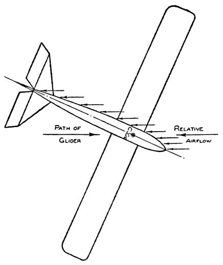
Fig. 11.—Directional or Weathercock Stability.
