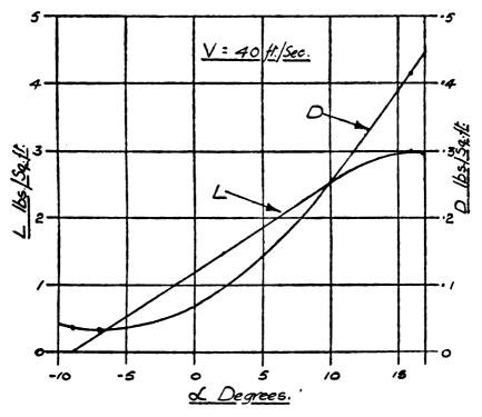
Fig. 5.—Lift and Drag Forces on Wing.
