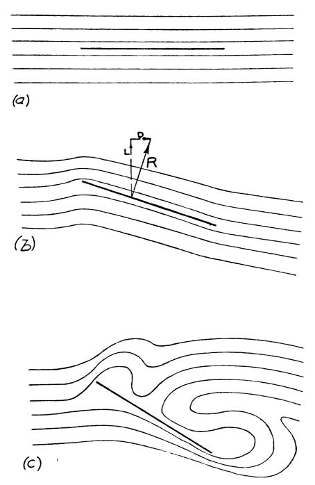
Fig. 2.—Airflow past Flat Plate.
