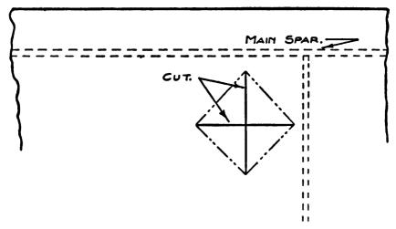
Fig. 43.—Opening up Fabric for Wing Repair.
