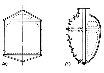
Fig. 35.—Construction of Fuselage Frames.
