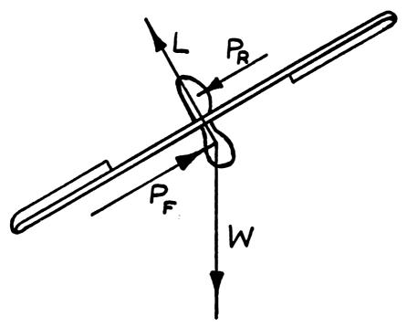
Fig. 24.—Forces Acting in a Sideslip.
