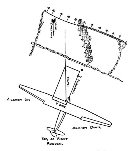
Fig. 27.—Landing Approach by Means of Sideslip.
