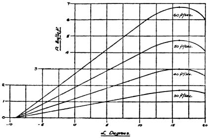
Fig. 4.—Air Reaction on Wing at Various Speeds.
