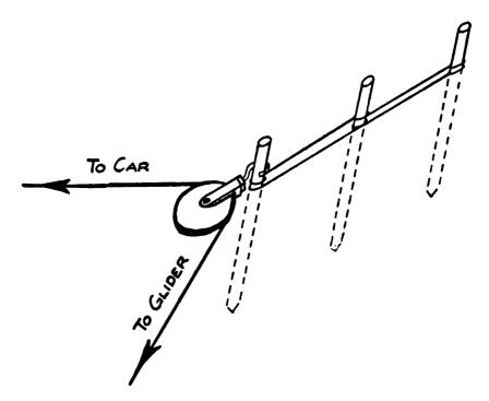
Fig. 29.—Pulley Fixture for Auto-Launching.
