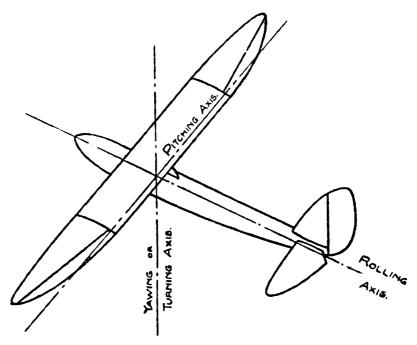
Fig. 9.—Axes of Movement.
