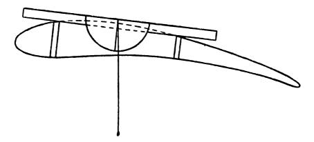
Fig. 15.—Incidence Board.
