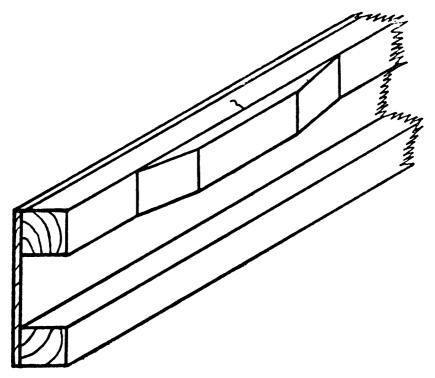
Fig. 40.—Spar Repair.
