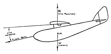
Fig. 7.—Forces on Glider in Normal Flight.
