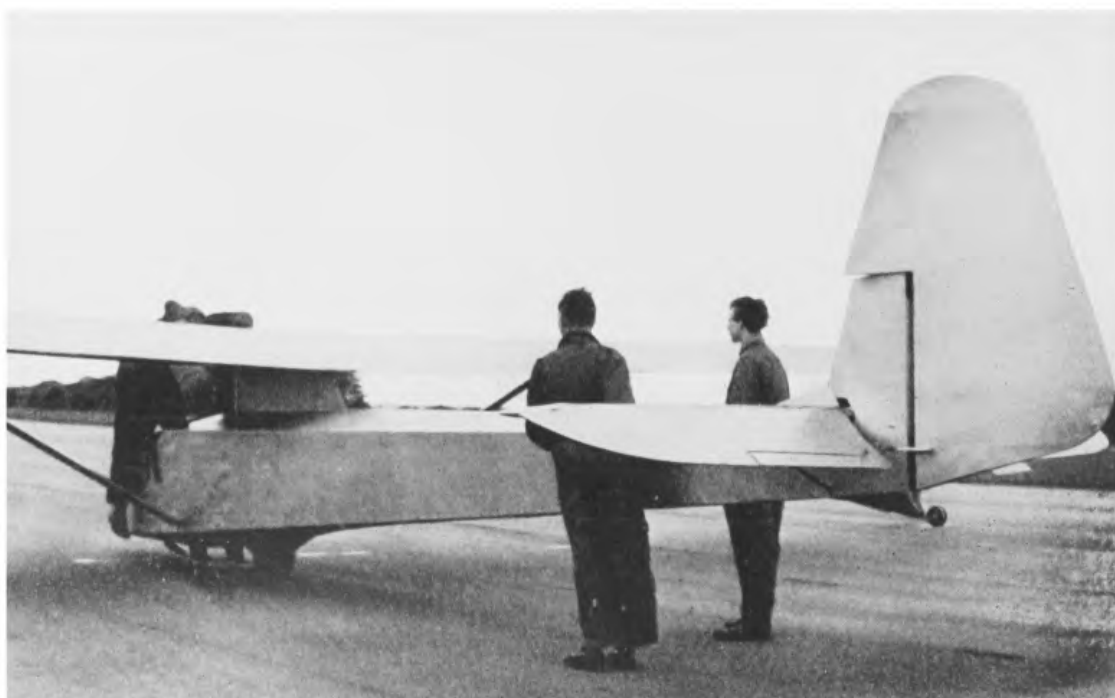
28. Before the pilots are in the cockpit, the tail must be held high if the glider is facing the wind. This will prevent it being blown over.
