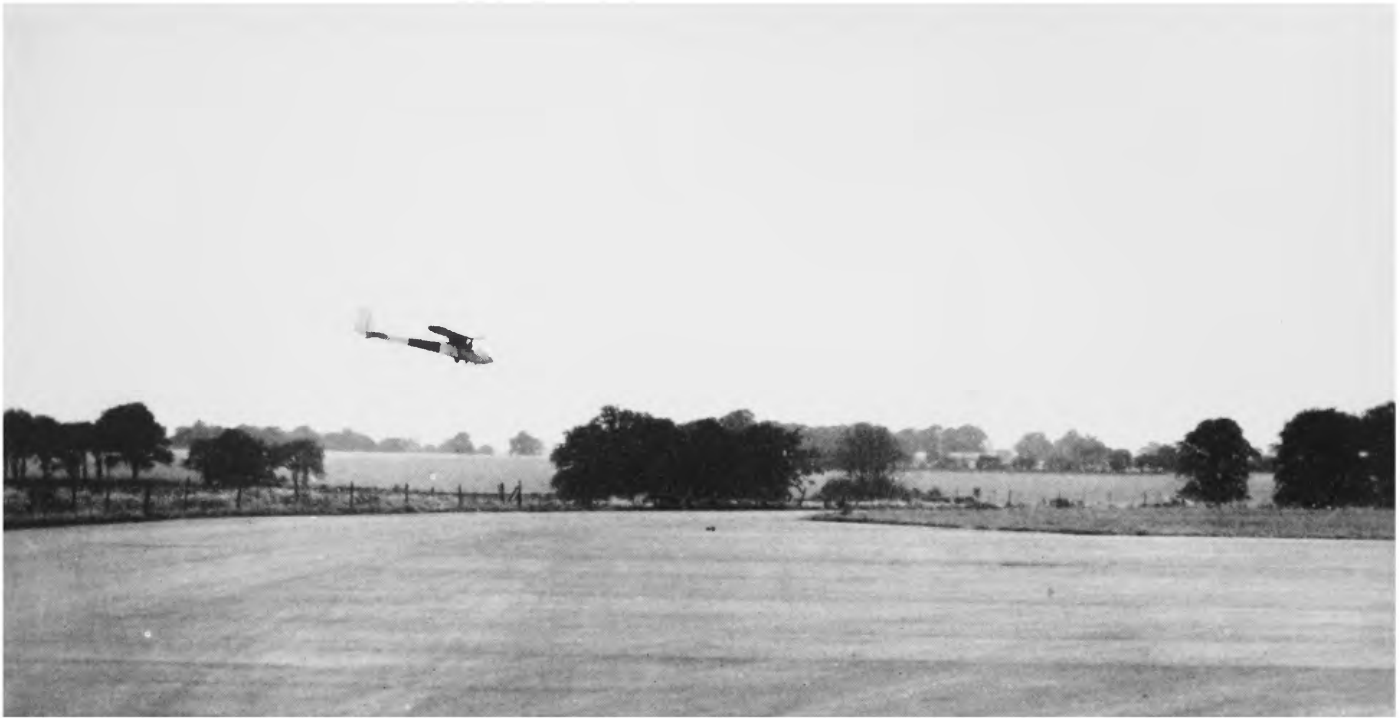
67. The Slingsby T21b, or Sedburgh as it is called by the A.T.C., is known all over the world as an excellent school two-seater. Here is 'Fanny' making a good approach to land at Lasham on a routine flight. The height over the fence, and the speed as shown by the nose-down attitude, are about right.
