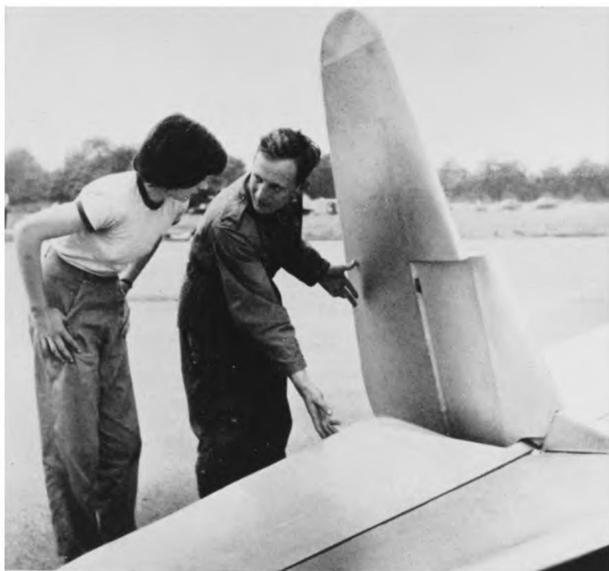
68. The first lesson. Instructor Brian shows 14-year-old Sarah the tail control surfaces, and how they move. The elevator which controls the speed is the horizontal surface which is moved up and down by the control stick. The rudder, which helps you to turn smoothly, is the vertical surface, and is controlled by rudder pedals.
