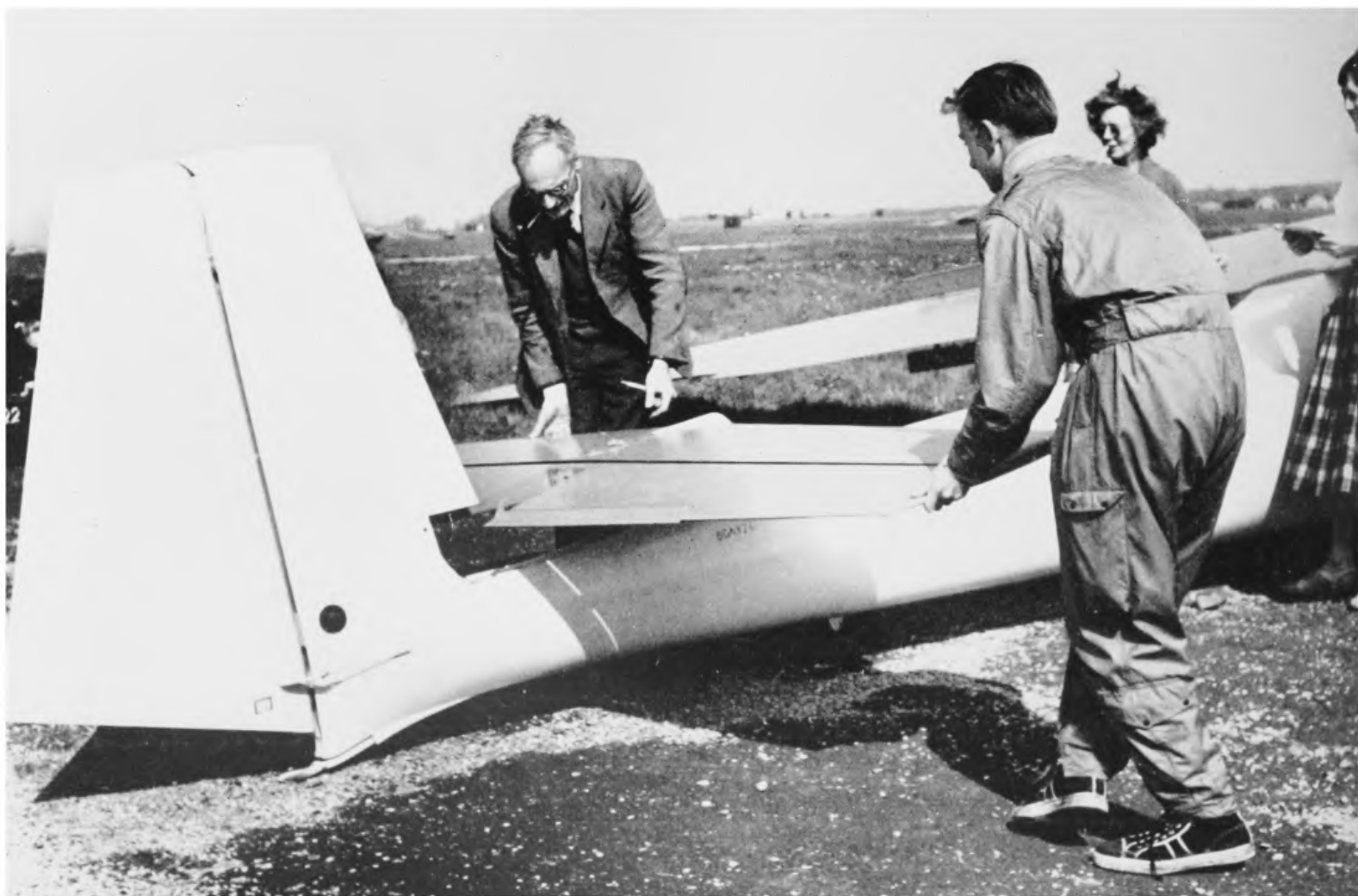
7. Now for the tailplane. Philip and Bob lower this carefully into place. They will screw down the special holding nut and then connect the elevator control. Before take-off the pilot must always check his controls, as a final safeguard against forgetfulness.
