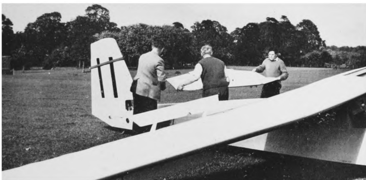
95. In one minute the tailplane is off, and on its way to its special rack in the trailer.
