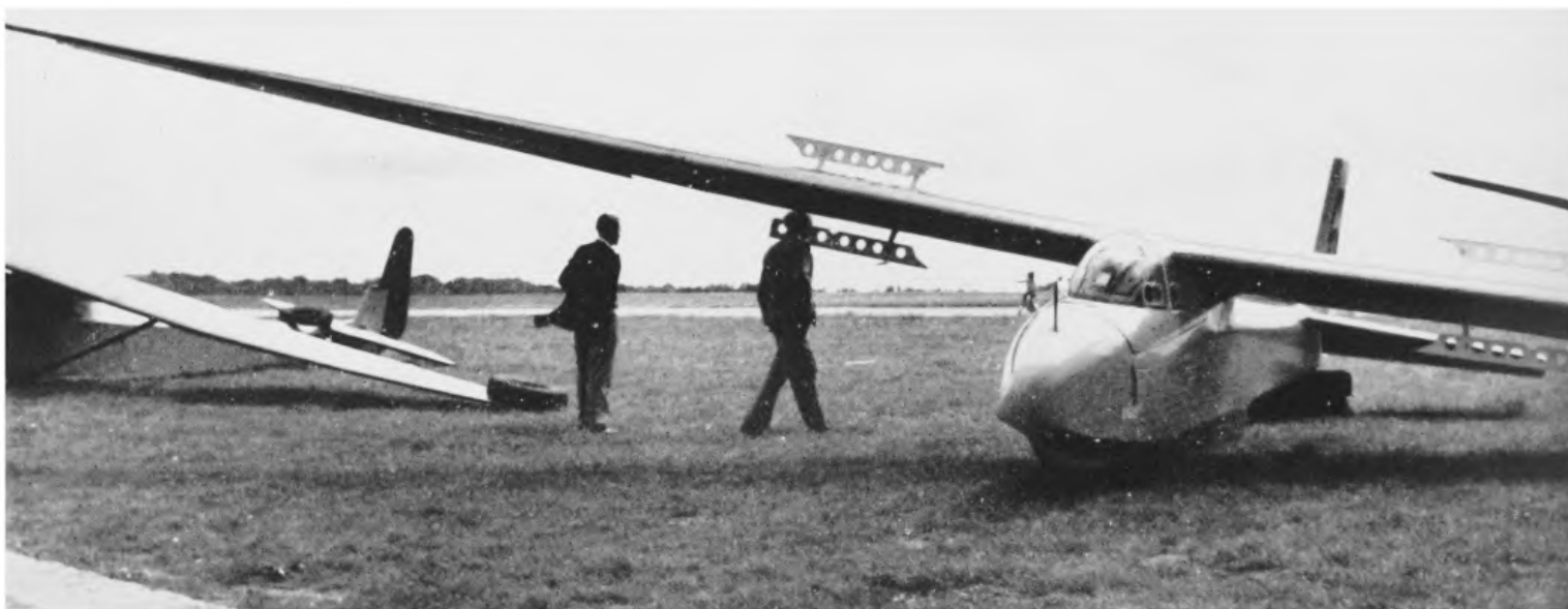
32. In order to steepen the approach path when coming in to land, the glider is fitted with air brakes, as shown on the Eagle. During flight they are totally enclosed inside the wings, and are extended by the pilot when he wants to land. Many air brakes limit the top speed of the glider, so that should the pilot get out of control in cloud, he can open the brakes, and this will prevent the glider going beyond its maximum permitted speed.
