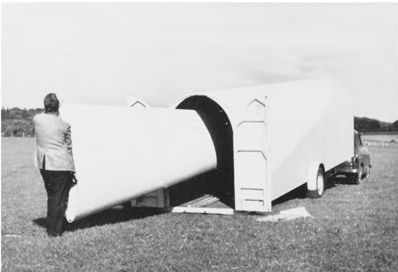
98. The wing is in three pieces. Only five minutes have gone by, and most of the glider is inside. Surprisingly, there is still room for the fuselage.
