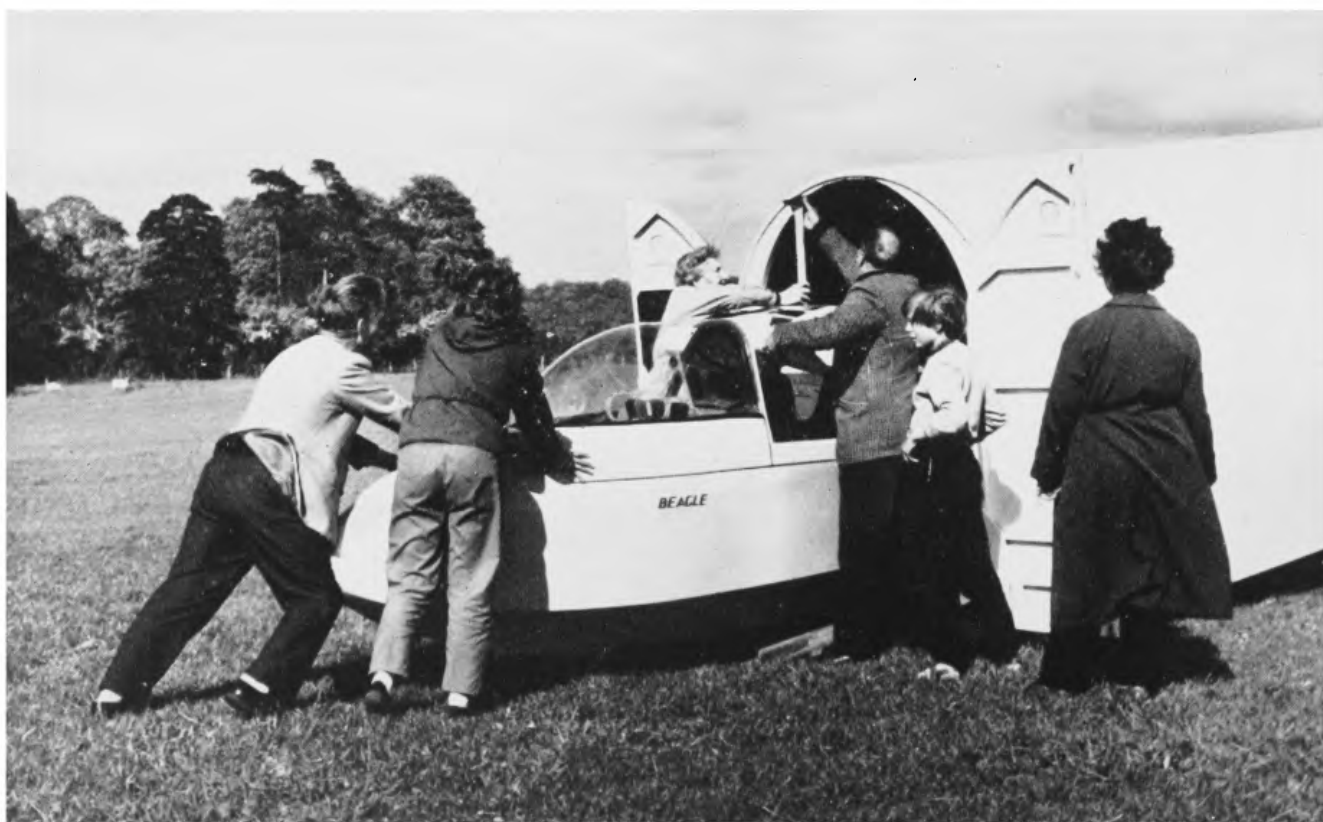
99. The tail-skid slides in along tram lines, the vertical support has tracks too. Seven minutes have gone by, and one minute is left to shut the doors, and have a good look round and see that nothing has been left behind.
