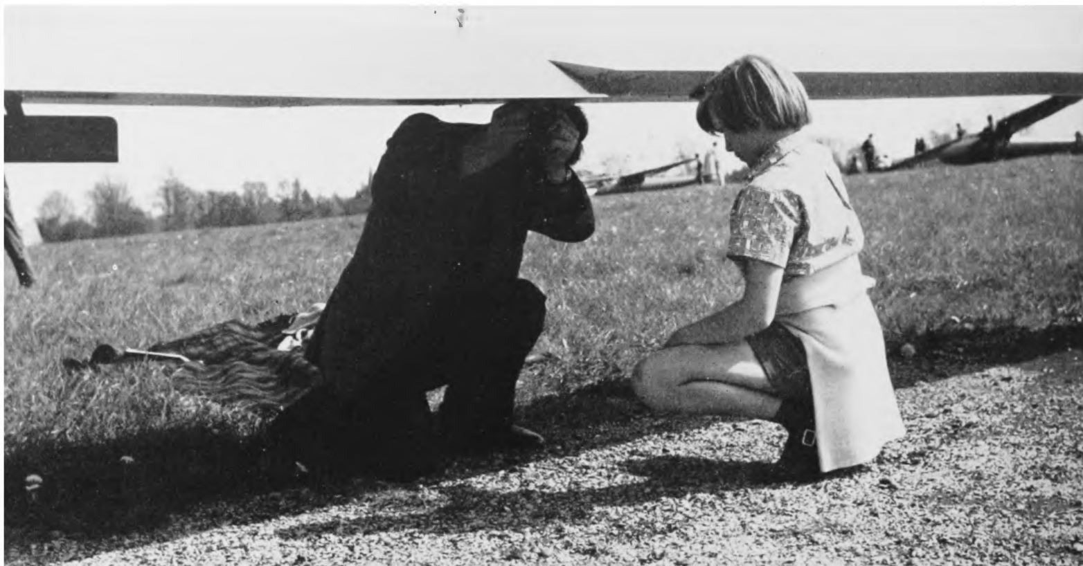
6. After the main pins have been put in they are secured with special safety pins. The handle on the top of the wing has been used to push the main attachment pin home. It will be removed before flight, and then kept in the glider. In this picture Philip is connecting the aileron control.
