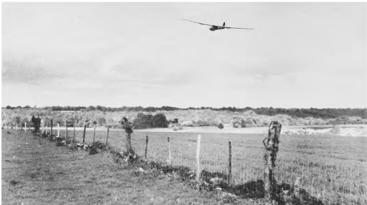
86. No luck, so the glider is turned towards the chosen field. As it is so small, the pilot must come low over the fence, at just the right speed. The air brakes are open to steepen the glide and the aircraft is coming straight towards the field, without having to do any further turns.
