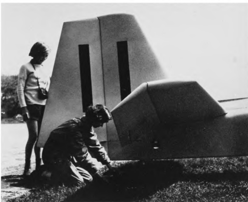
74. Even with the wing weighted down, the glider has a tendency to weathercock its nose into wind in gusts, so another tyre is placed on the ground to the lee, or downwind side of the tail skid, so that it will not be able to swing.
