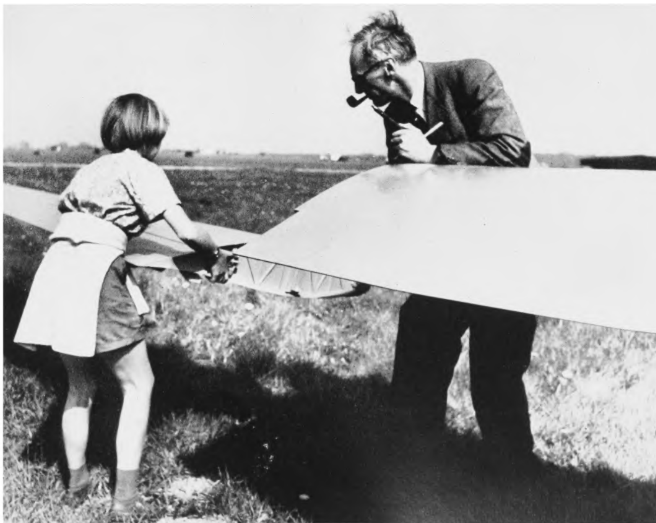
5. Now the port outer panel. The span of the Skylark II is 48 ft. and the whole glider can be rigged in less than ten minutes. It has no struts or wire bracing, but is strong enough to be flown safely in the violent turbulence of big thunderstorms.
