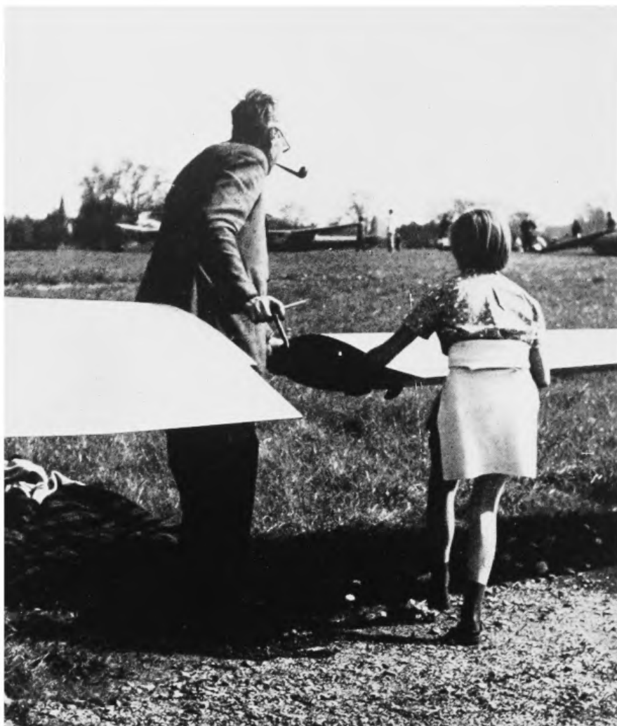
4. Philip and Elizabeth are attaching the starboard outer panel. This is fixed into place with the steel pin in Philip's hand.
