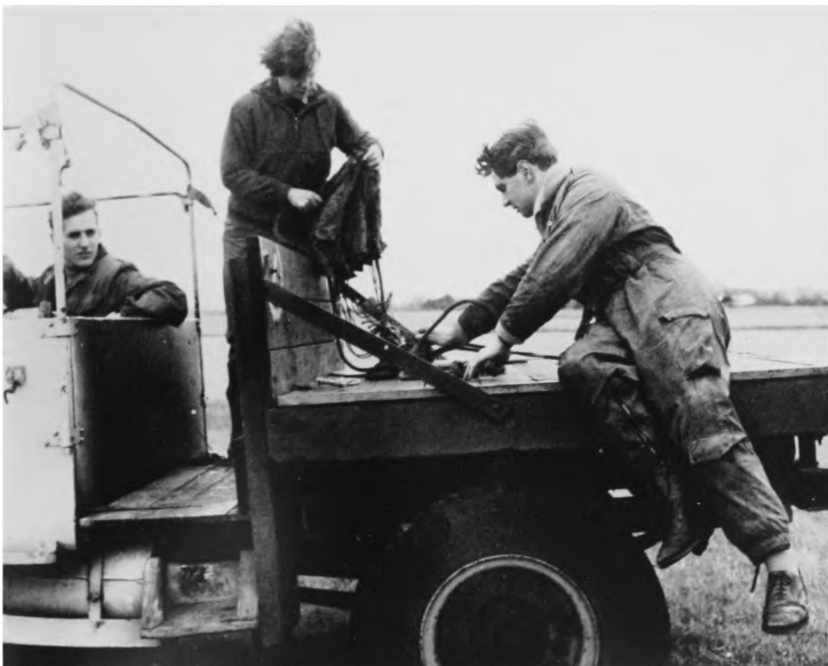
49. The tow car, having given a launch, drops the end of the cable, and then returns up the runway to take the glider end back to the launch point. Here it is being hooked on to the car release, while the parachute, which allows the wire to fall gently and straight after the launch, is inspected.
