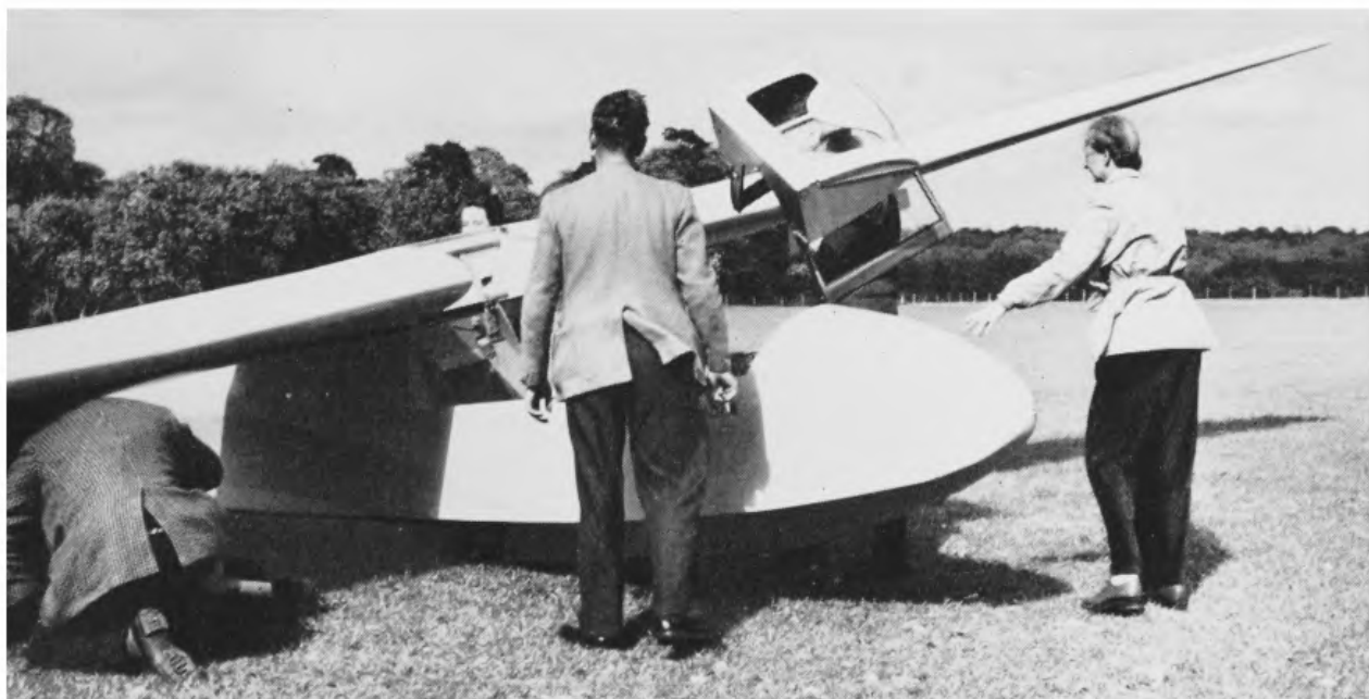
96. The cockpit cover comes off, aileron and air brake control disconnected. All the partners know the drill, so work proceeds smoothly.
