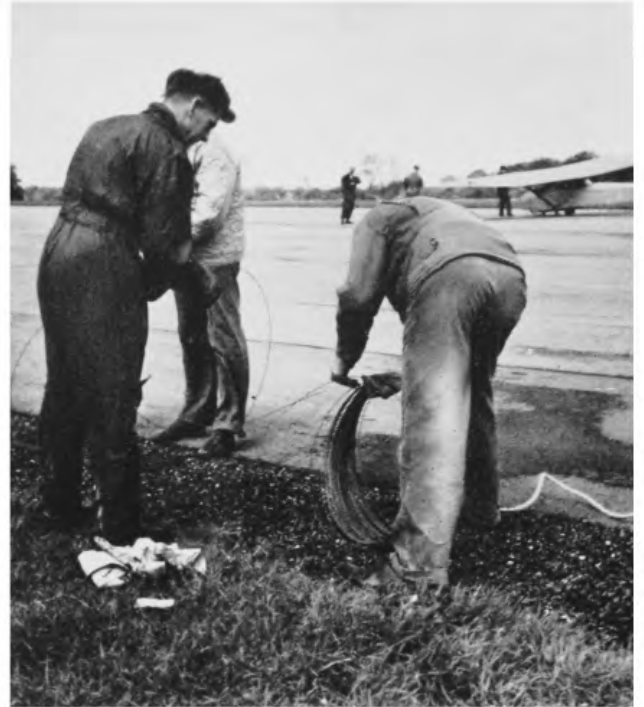
47. Now let us return to the launch point to see how the glider, so remote from the winch or tow car, is got off the ground. Cables from a two-drum winch have been towed out. The driver has followed a straight line to the launch point so that the cables will not be twisted, and care is taken that they are used in a pre-arranged order, so that the winch-driver will not pull in a cable which is not attached to a glider. Spare cables must never be held, or even touched, while launching is in progress.
