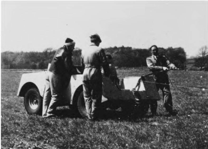
47. Now let us return to the launch point to see how the glider, so remote from the winch or tow car, is got off the ground. Cables from a two-drum winch have been towed out. The driver has followed a straight line to the launch point so that the cables will not be twisted, and care is taken that they are used in a pre-arranged order, so that the winch-driver will not pull in a cable which is not attached to a glider. Spare cables must never be held, or even touched, while launching is in progress.
