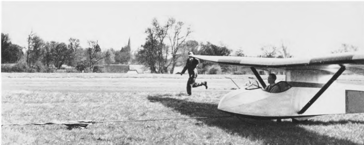
31. Because a glider has only a single landing wheel, it sits on the ground with one wing down. When the glider is about to take off, the wings are held level, until it has got enough speed for the controls to become effective.
