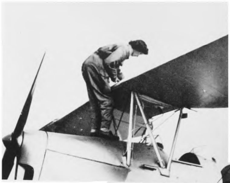
63. The aeroplane, too, is looked after and refuelled by members. First of all, Anne takes off the filler cap, and then guides the hose . . .
