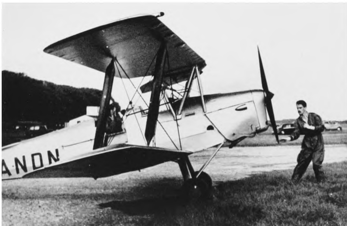
65. With the tug pilot in the cockpit, and chocks in front of the wheels, the prop is swung, and the Tiger Moth will then be taxied out to tow up the gliders waiting to fly.
