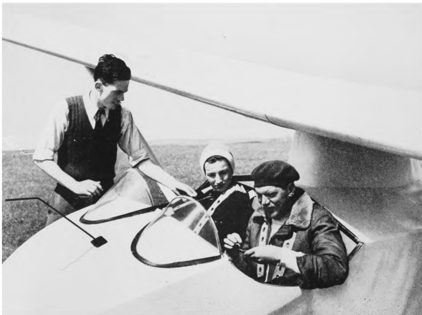
14. This is the cockpit of a T21b school two-seater. It is open so that the pupil will be able to feel the airflow on her face, and learn quickly how to correct for change of speed, or when she is skidding through air instead of turning accurately. The pupil has a good view, and is taught to keep a proper look out for other aircraft.
