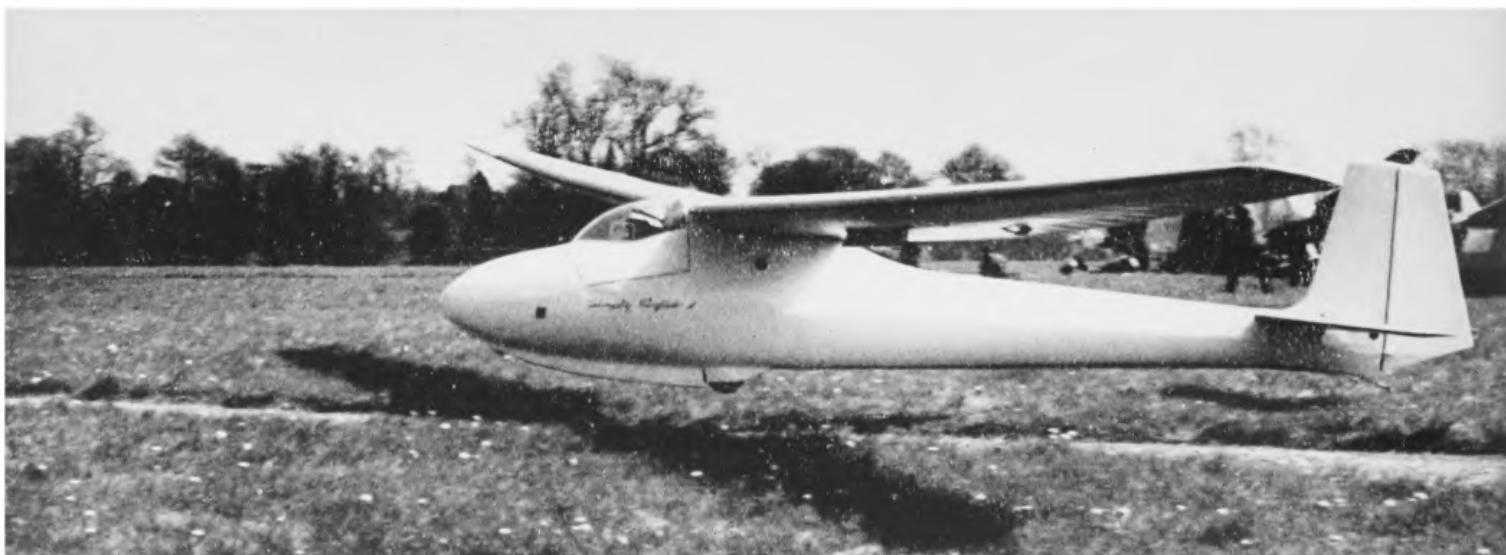
33. Philip just about to land in the Skylark II. The air brakes are extended, and the glider is about to touch down on the main wheel and tailskid at the same time—an excellent two-point landing.
