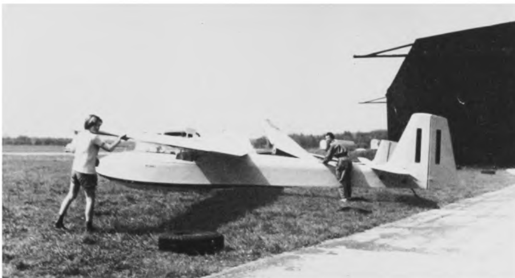
72. Learning to glide is not all flying, for although gliders are extremely strong in the air, they are easily damaged by gusts of wind on the ground, and must be parked properly. The glider has been brought from the hangar and is parked with the air brakes open and one wing pointing into the wind.
