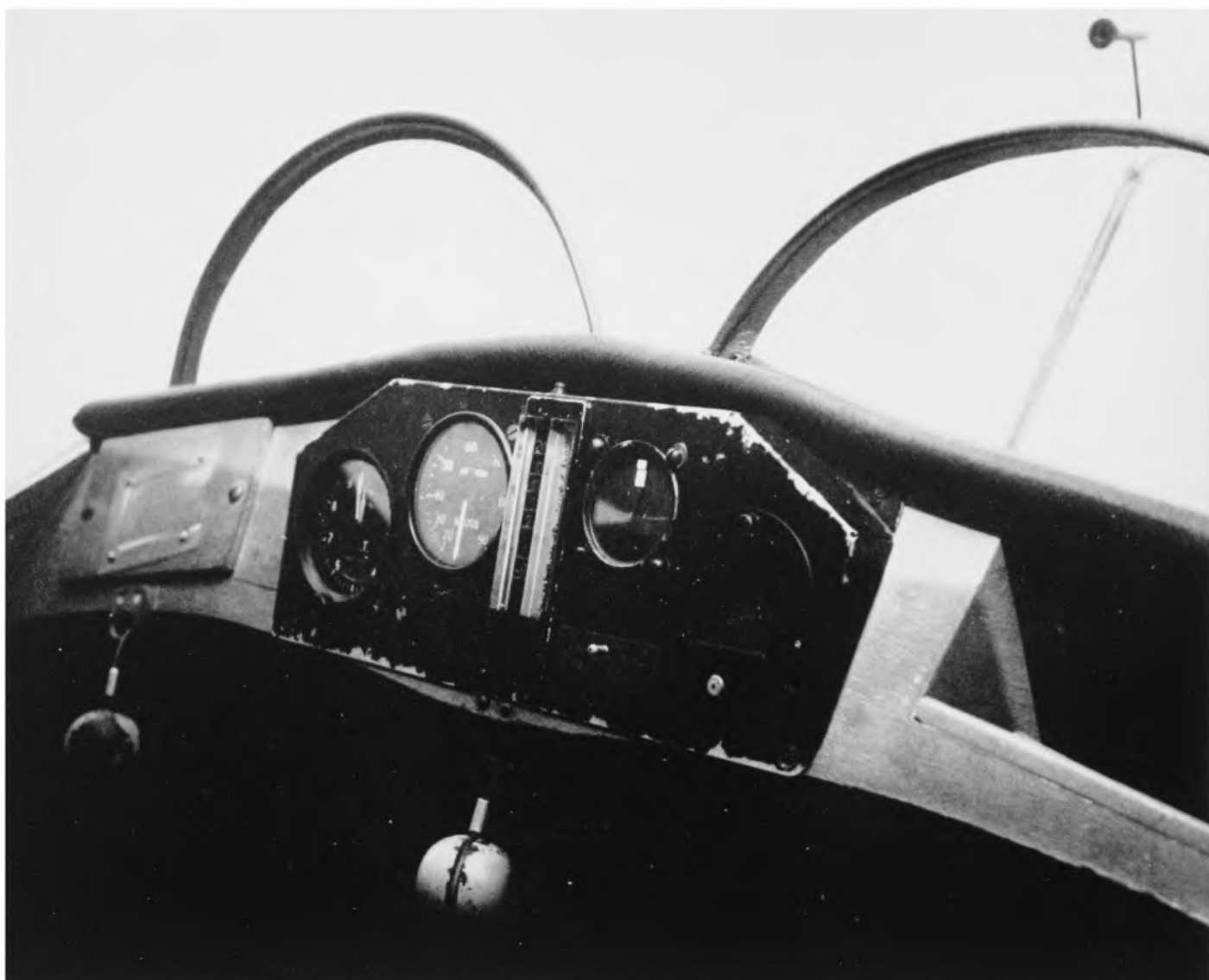
71. The instrument panel of the much-used school two-seater. The aircraft has full dual control, and so both the instructor and pupil have their own cable release knob. The central vertical instrument is the Variometer which tells the pilot whether the glider is flying in rising or sinking air. Immediately to its left is the Airspeed Indicator in knots, and left again, the Altimeter. On the right of the Variometer is the Turn-and-Slip Indicator for cloud flying, with its battery switch below. On the extreme right, but barely visible, is the Compass.
