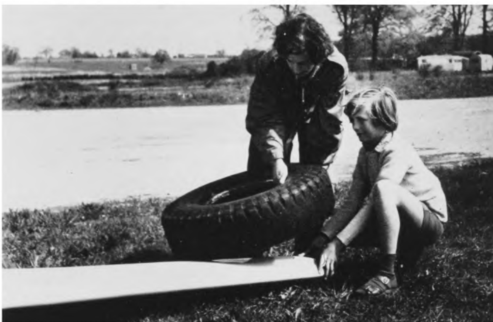
73. This windward tip is put carefully on smooth ground and a heavy tyre placed on it. Two tyres may be necessary if the wind is strong.
