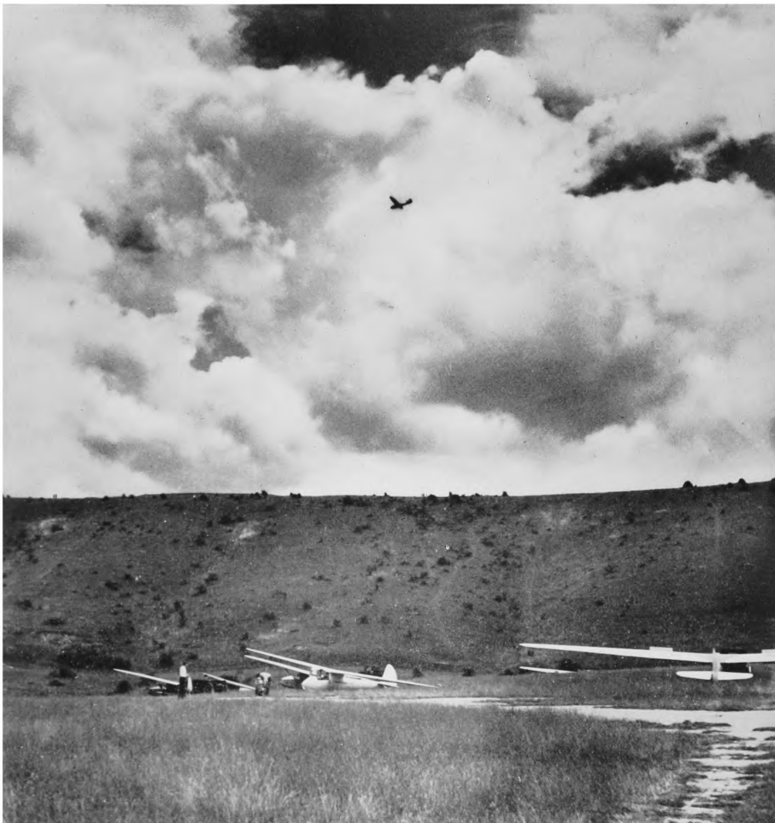
39. Hill soaring can also be used as a way of jumping-off on a cross-country flight on thermals. The pilot gets into the clear fresh air above the ridge and waits until the cloud of his choice comes along.
