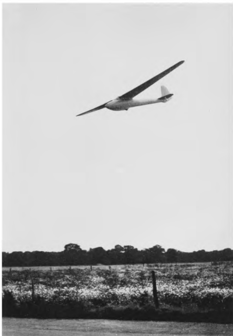
29. When a glider is approaching to land it must increase speed. This nose-down attitude can be seen as the Olympia comes in.
