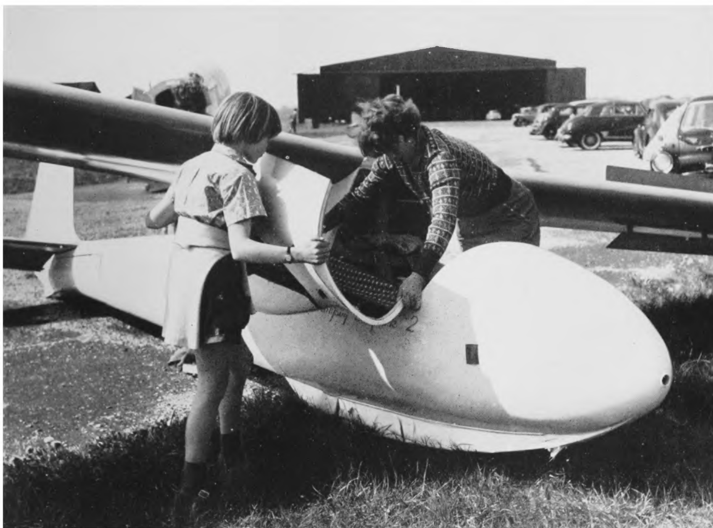
8. Finally the canopy, which was removed while the glider was being rigged, is attached, and 8\frac{1}{4} minutes after the trailer doors were opened the glider is ready to fly.
