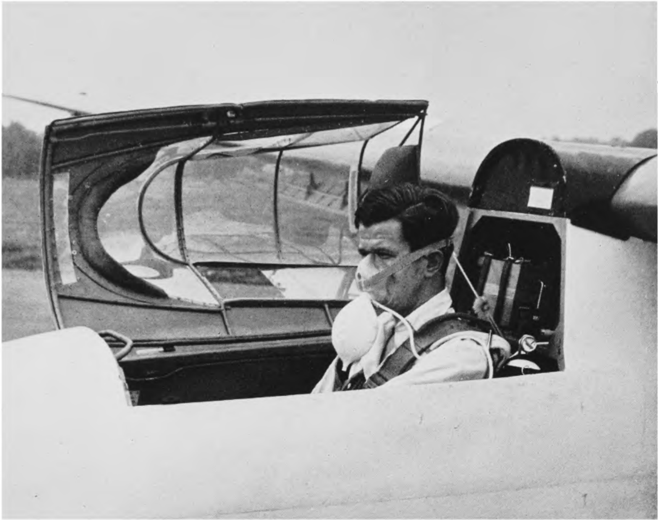
21. Doug. checks the lightweight oxygen before take-off. If he goes above 15,000 ft. he will need it, as there will not be quite enough for him in the rarefied air high up. The 240-litre bottle is stowed behind his shoulder, and the gauge indicates full.
