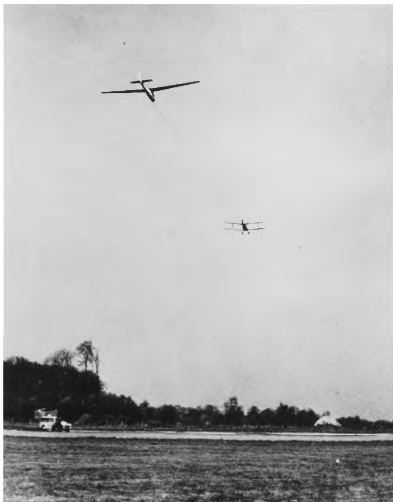
62. Aero towing is a safe and easy way of launching gliders, and one which can take the glider to areas of good upcurrents. After a cross-country flight, the glider can be towed home again if it has been landed on an aerodrome or large field.
