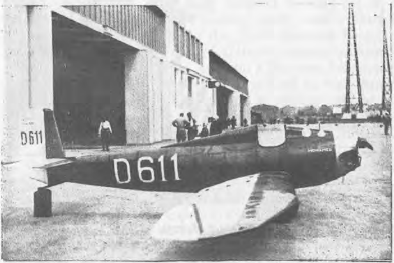
24. THE DARMSTADT ACADEMIC FLYING GROUP'S "MOHAMED," A TYPICAL DESCENDANT OF THE SOARING PLANE FITTED WITH A LIGHT ENGINE
