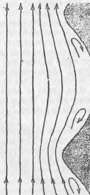
WINDWARD EDDY STEEPER SLOPES PRODUCE EDDIES TO WINDWARD AND TO LEEWARD
