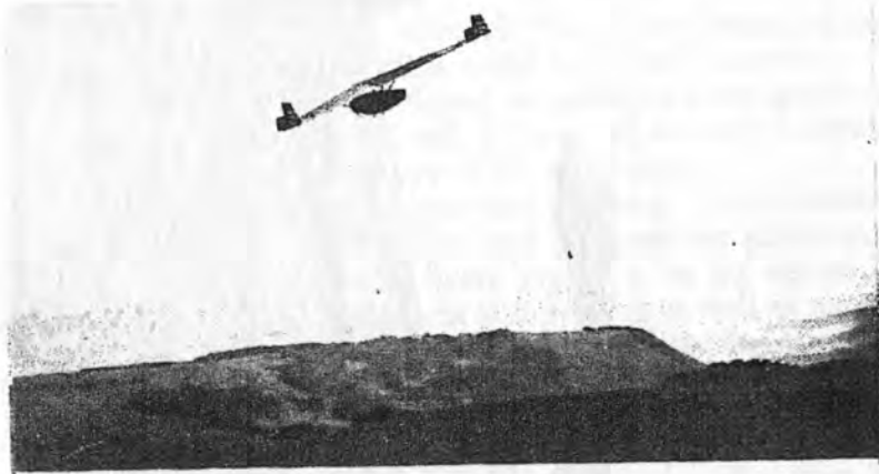
4. THE RHÖN-ROSSITTEN COMPANY'S TAILLESS SOARER, THE "STORCH," WHICH WAS GIVEN A LIGHT ENGINE FOR A SERIES OF EXPERIMENTS
