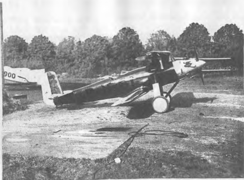
23. THE DARMSTADT ACADEMIC FLYING GROUP'S D.18. FUSELAGE AND WINGS SHOW THE EFFECT OF THE EXPERIENCE GAINED IN SOARING FLIGHT
