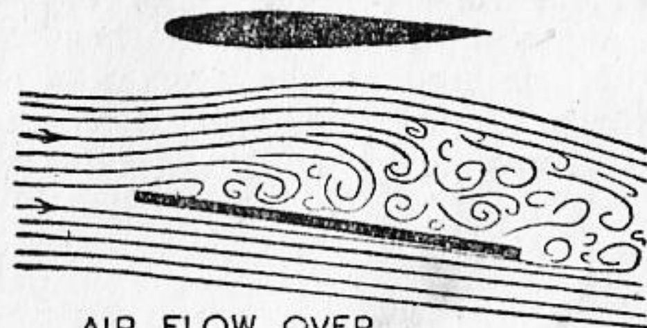
AIR FLOW OVER FLAT SURFACE
