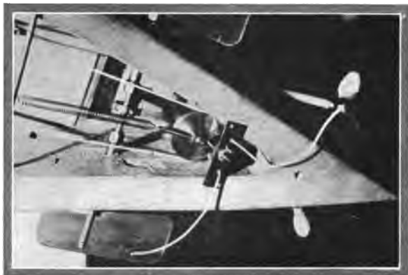
Fig. 208—The rudder control mechanism
