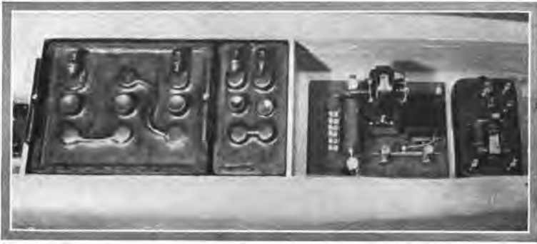
Fig. 200—The storage batteries and central control mechanism
