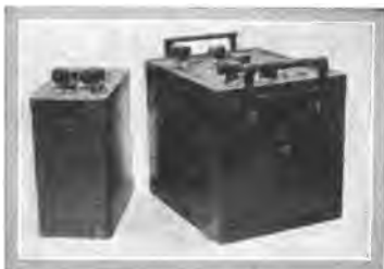
Fig. 198—The storage batteries used on the submarine
