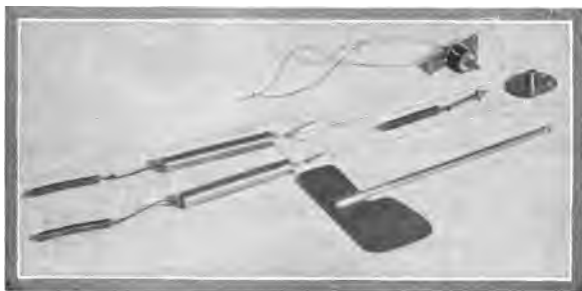
Fig. 209—The parts of the rudder control mechanism
