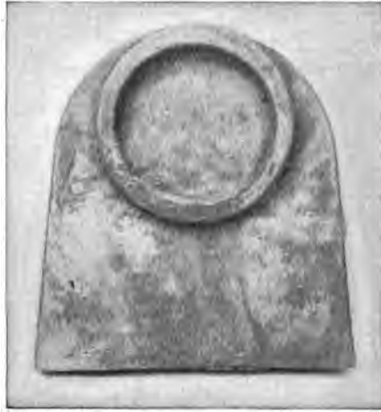
Fig. 151—Casting of a waterback
