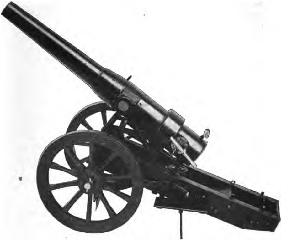
Fig. 300—The model siege gun completely assembled and elevated at 45 degrees
