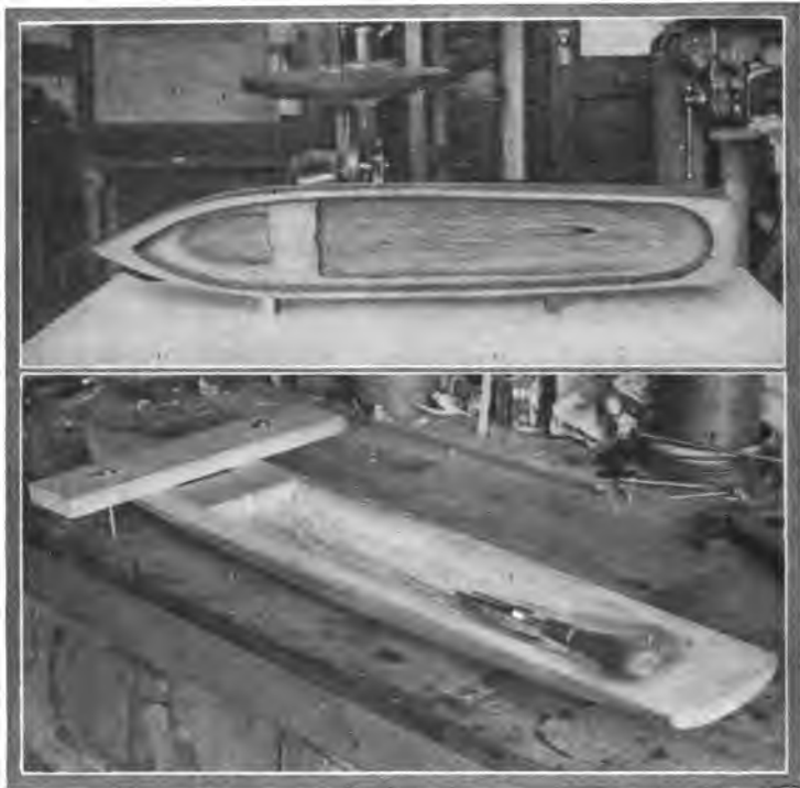
Fig. 190—How the boards that compose the boat are gouged out. The complete hull is shown above
