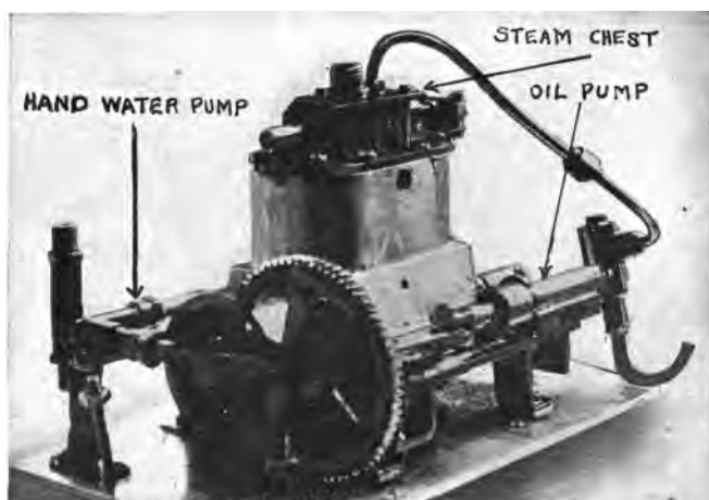
Fig. 168—The engine, showing the hand water pump and the oil pump
