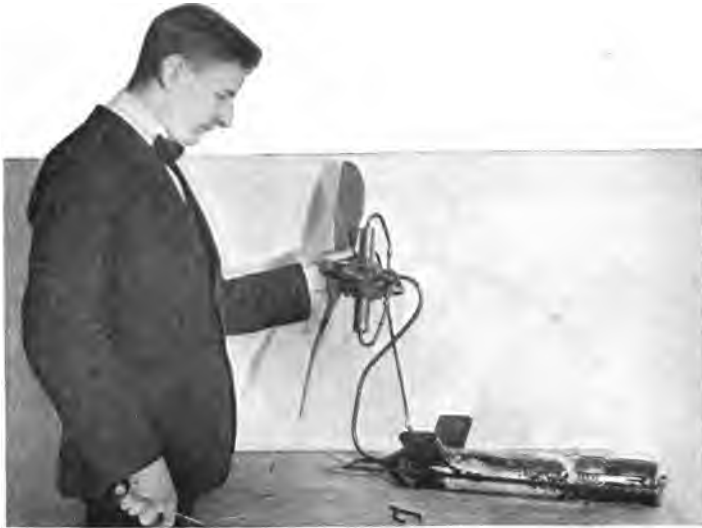
Fig. 117—The four-cylinder engine and its flash boiler
