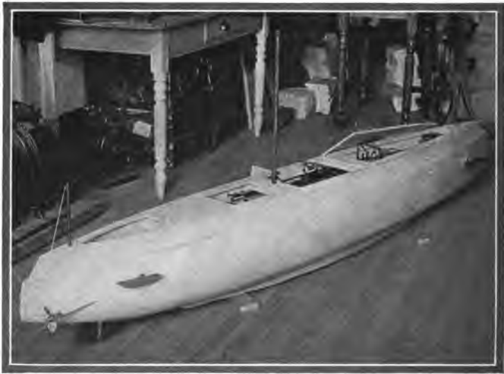
Fig. 223—The submarine with the deck removed
