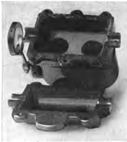
Fig. 101—The crankcase of the engine after being machined
