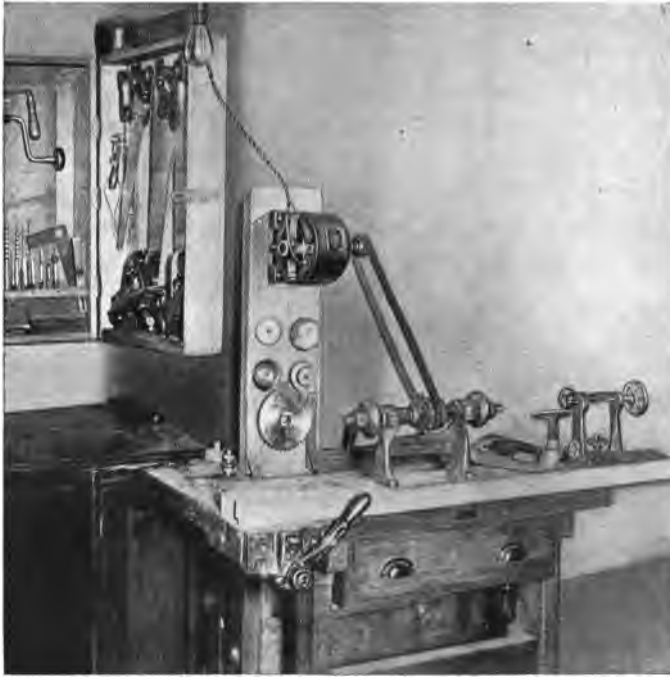
Fig. 6—A power-driven lathe mounted on a work bench
