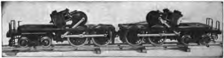
Fig. 280—The locomotive chassis, showing the driving motors and the method of gearing them to the drivers
