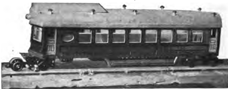
Fig. 288—The model gyro-car balancing itself upon a single rail
