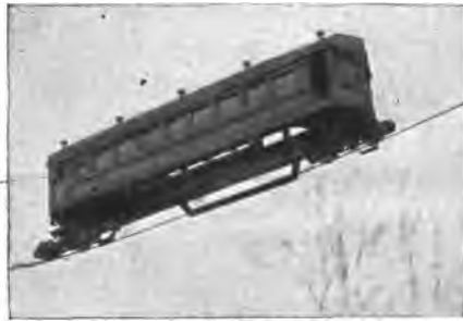
Fig. 287—The model gyro-car balancing itself upon a wire
