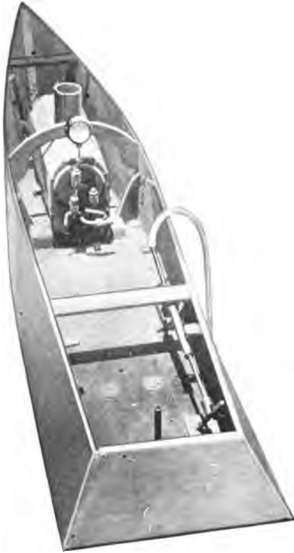
Fig. 179—The boat with the deck removed. The hand water pump is shown at the right
