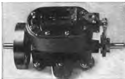
Fig. 99—Top view of the engine showing the steam chest uncovered
