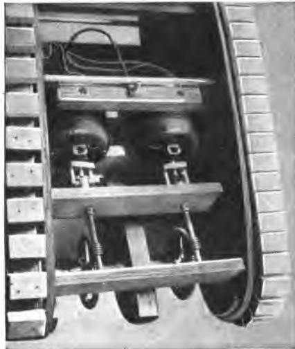
Fig. 296—The rear of the tank with the cover removed to show the mounting of the driving motors
