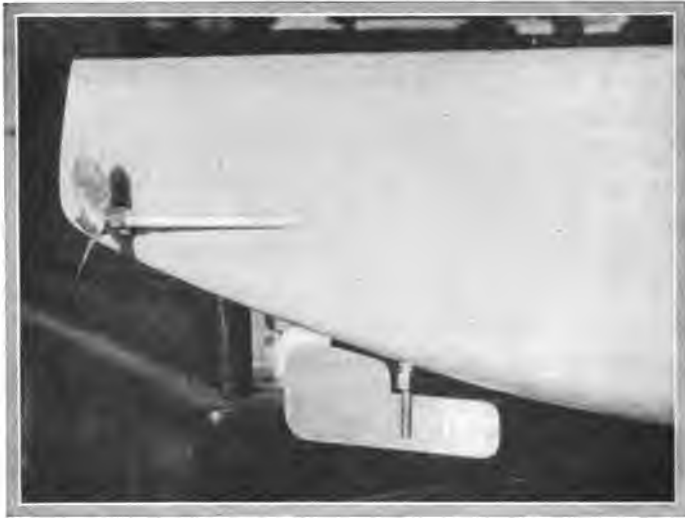
Fig. 207—The stern of the submarine hull, showing one of the propellers and the rudder
