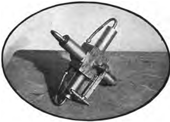
Fig. 116—The four-cylinder steam engine assembled
