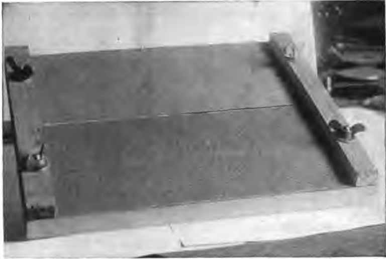
Fig. 59—A lap board which is very convenient for polishing and grinding flat surfaces
