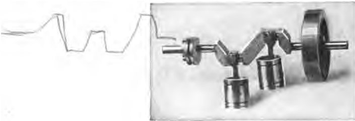
Fig. 98—The completed crankshaft for the engine, with flywheel, pistons and eccentric mounted in place
