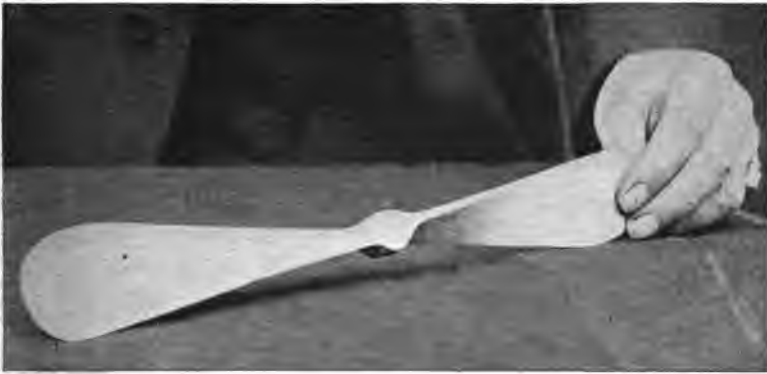
Fig. 274—Aluminum aerial propeller constructed for use with the engine
