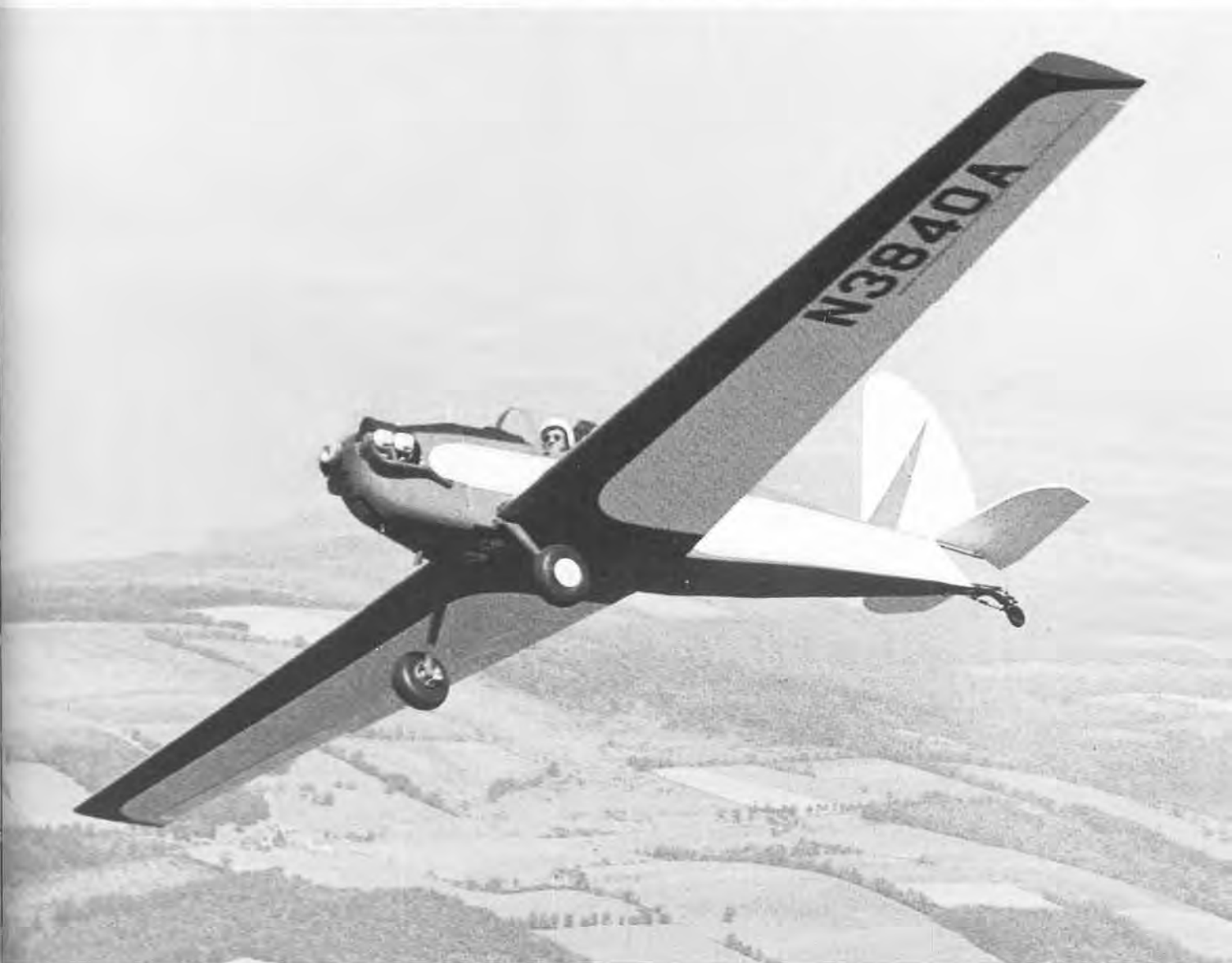
The SA 1-30 aeroplane used 1-26 wings and tail unit, and had a sprung landing gear.
