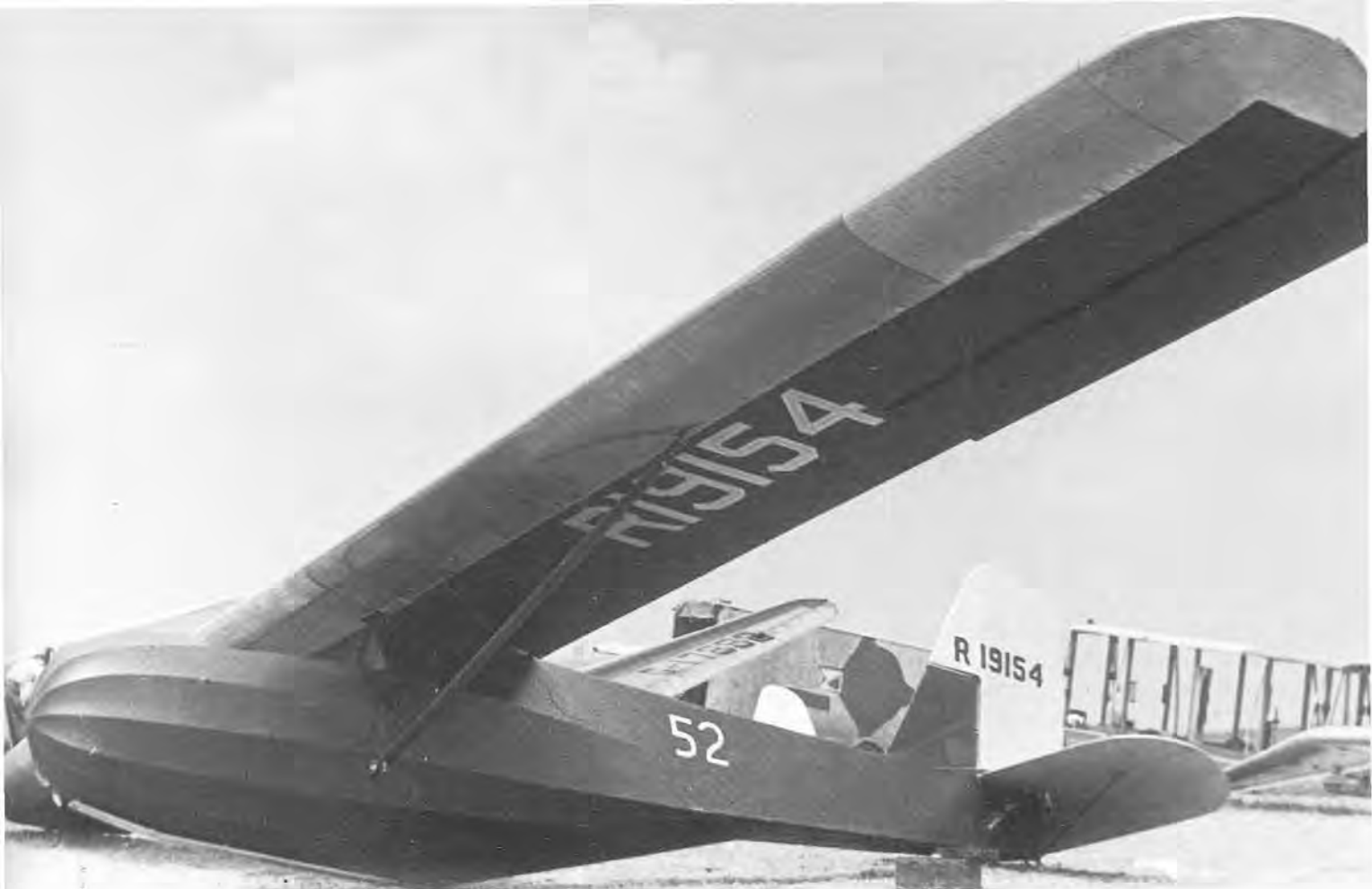
ABOVE: The SGU 1-7 at the 1937 Nationals. Note the angular rudder; later replaced.
