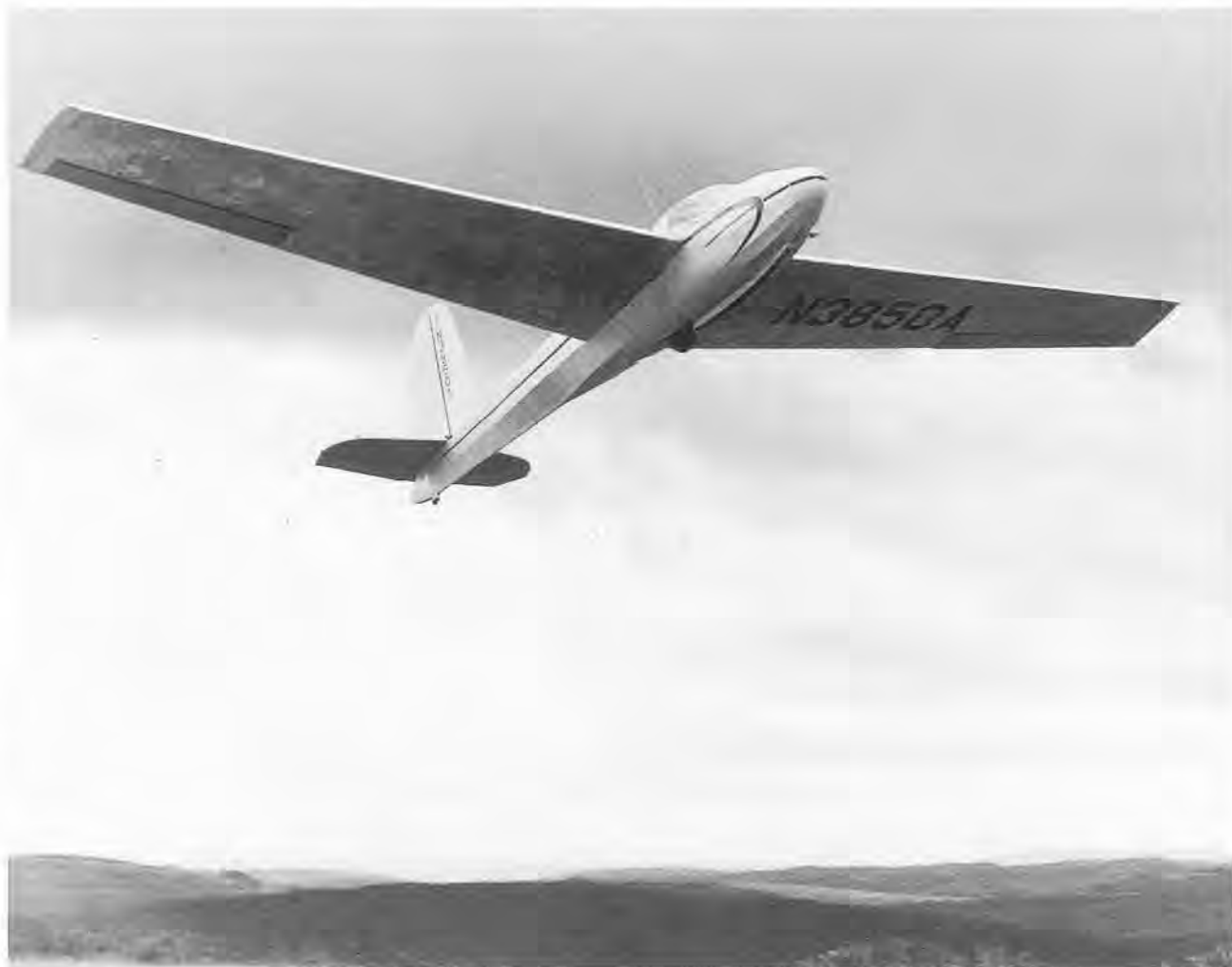
An SGS 1-26 with the original fabric-covered nose section takes off on winch launch.
