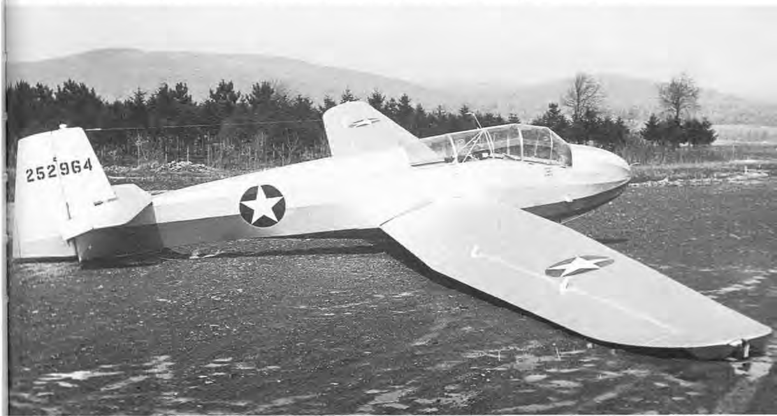
A typical production TG-3A outside the new Schweizer plant. It was painted all silver except for the national insignia.
