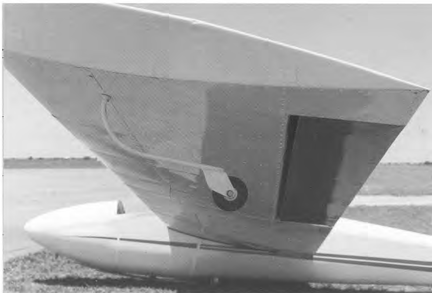
A 1-26B with the optional tip wheels used for training flights. (M. Simons)
