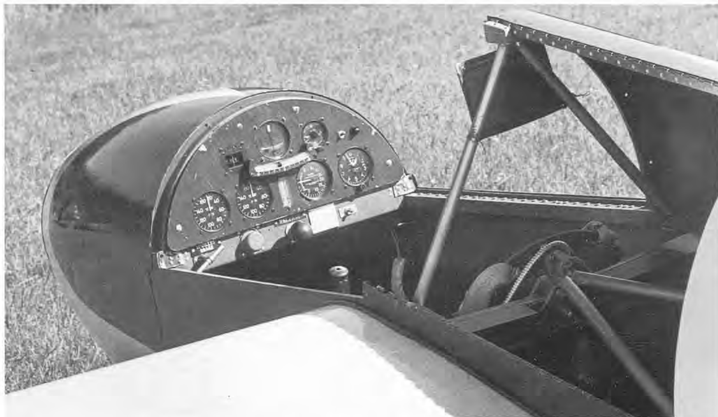
A fully instrumented 1-23D, with the side panel removed to reveal the crash pylon.
