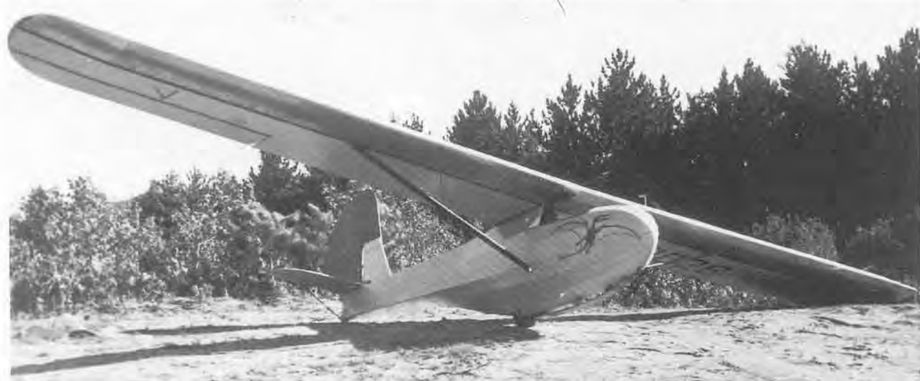
TOP: The fabric-covered, steel-tube-framed fuselage and the metal skinning of the wing leading edge are shown clearly here. ABOVE: The Altosaurus Soaring Club became our first genuine customer, taking delivery of the second SGU 1-7, which they named Pterodactyl . Note the revised rudder shape, which was also used on the prototype after some flying experience.
