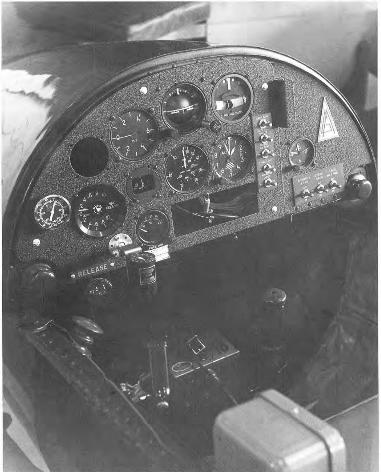
The instrument panel of the 'Sierra Wave' SGS 2-25. One instrument and the radio are missing.
