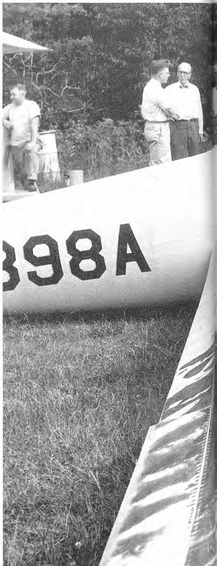
RIGHT: Another view of the original SGS 1-29 being prepared by flight crew for its first test flight. This angle shows the wing not yet filled or painted.
