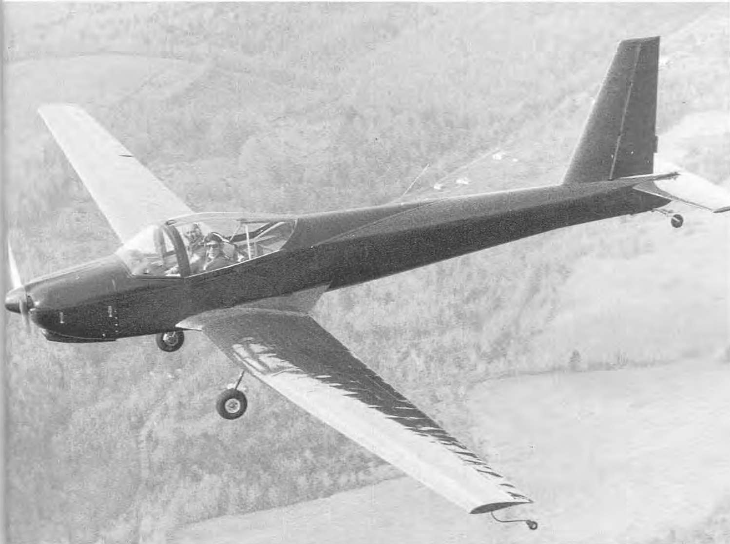
The prototype SGM 2-37 motor glider; built for the U.S.A.F. Academy. The rear fuselage and tail unit were from the SGS 2-32 sailplane, but note the absence of the dorsal fin extension.
