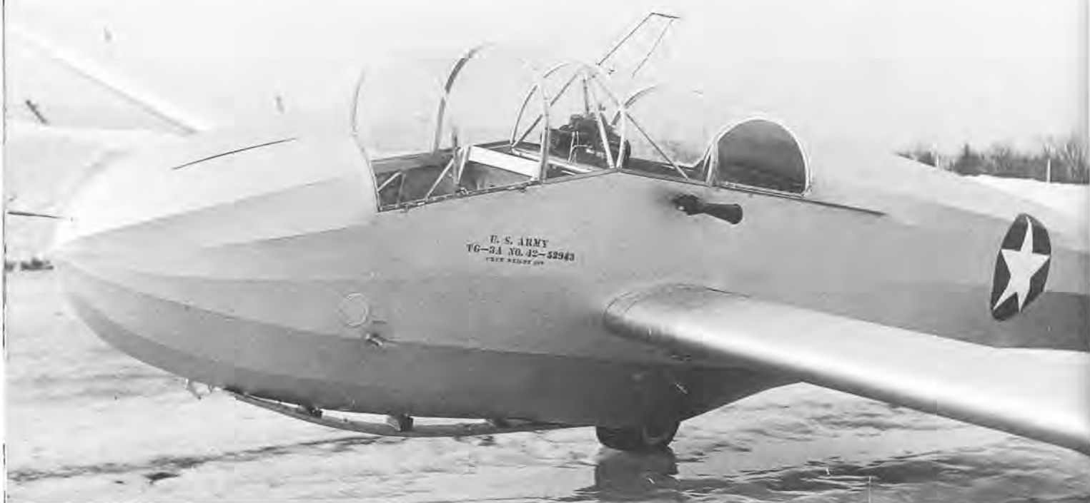
A production TG-3A, showing the stencilled markings required by the U.S.A.A.F. Note the step to help the front pilot to get into the cockpit. The large venturi was used to drive gyro instruments. Radio was sometimes carried, as revealed by the aerial.
