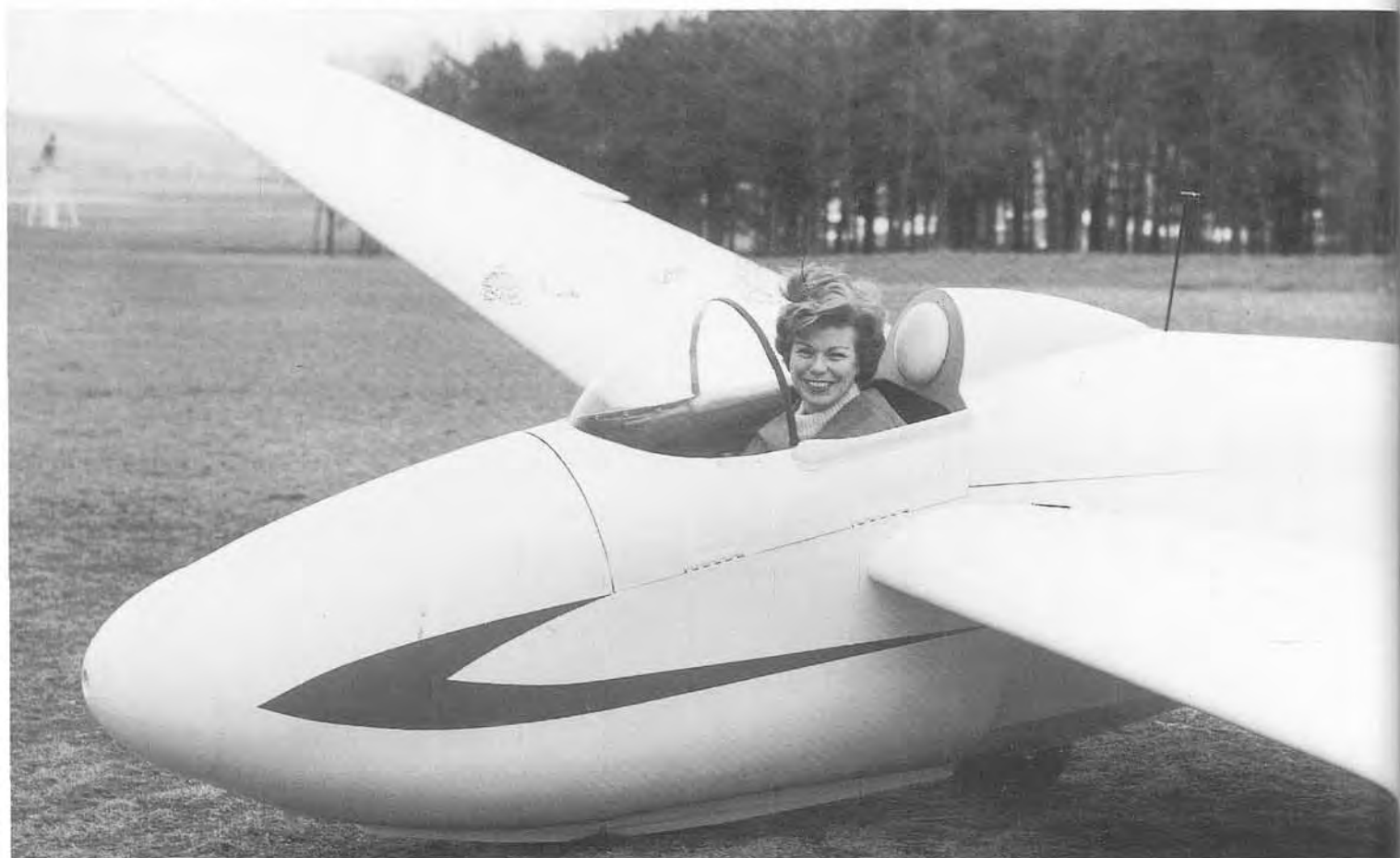
BELOW: For those who prefer to fly with an open cockpit, a 'sports' canopy is available for the 1-26.
