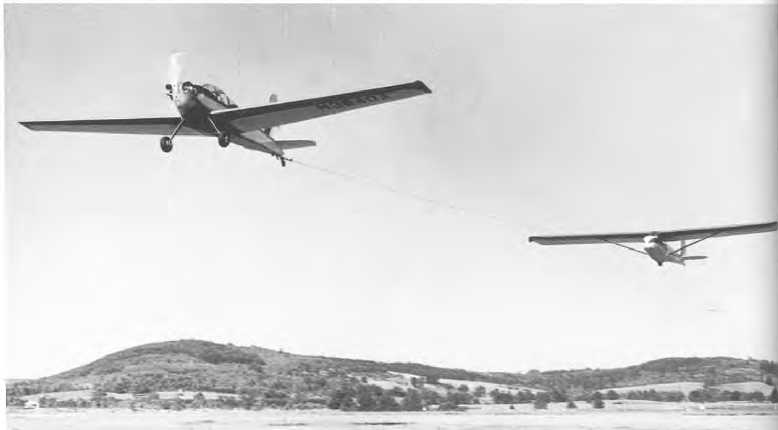
ABOVE: The 1-30 single place airplane ready for take off at Chemung County Airport. BELOW: The SA 1-30 made a satisfactory tug for relatively light sailplanes.
