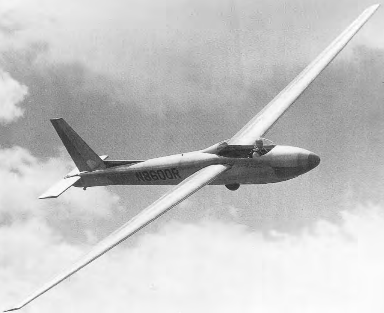
Bernie Carris test-flies the prototype SGS 2-32 with the original rectangular tailplane.
