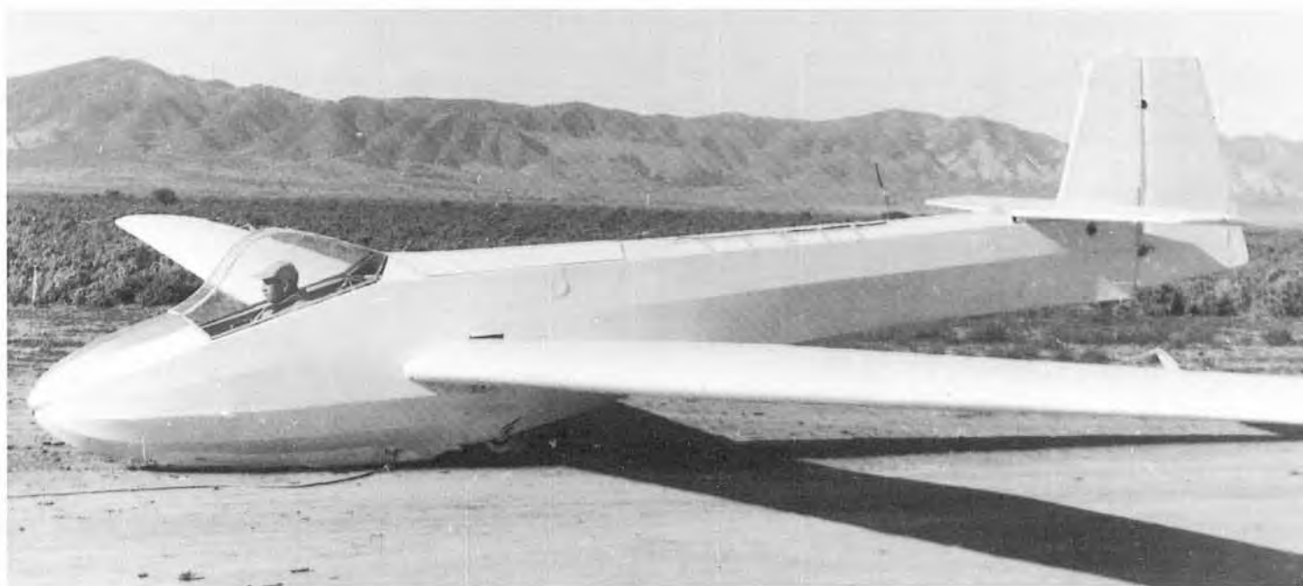
TOP: Paul Schweizer in front cockpit and Emil Lehecka in rear cockpit of No 114 commercial version of the TG-3A at Harris Hill. ABOVE: Examples of the TG-3 were to be found in many places around the world. This one was imported to Australia and modified to 'flat-top' configuration to reduce drag. It is here shown at the Port Augusta Gliding Club in South Australia. (Australian Gliding)
