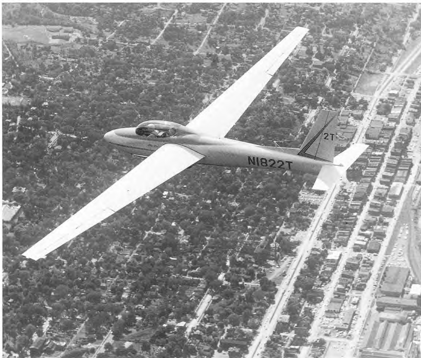
The Blue Bird SGS 2-32 over Corning, New York. Note the unusual aerial on the dorsal fin.
