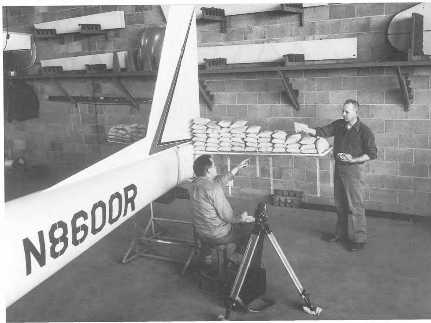
BELOW: Proof loading of the tapered tailplane of the 2-32. Ken Smith, the engineer, on the right, and Bill Solometo apply the loads.
