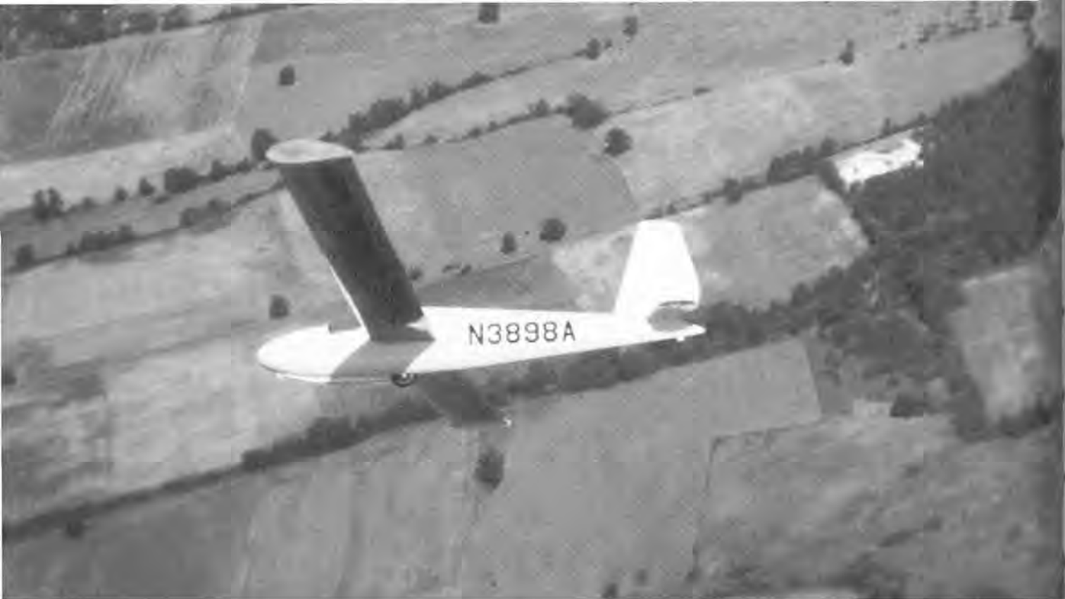
The SGS 1-29 circles, showing the tip plates on the wings which also acted as tip skids. The plates were later removed and the wingtips reshaped. A dorsal fin extension was also added.
