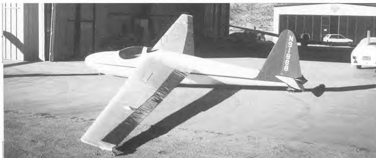
Top: The SGS 1-24 Brigadoon, now based at Tehachapi in California, showing the rear windows intended for the small passenger. Above: The 1-24 originally had fabric-covered areas on the wing, behind the rear spar. Soon after the move to California these panels were covered with metal for better resistance to the sun.
