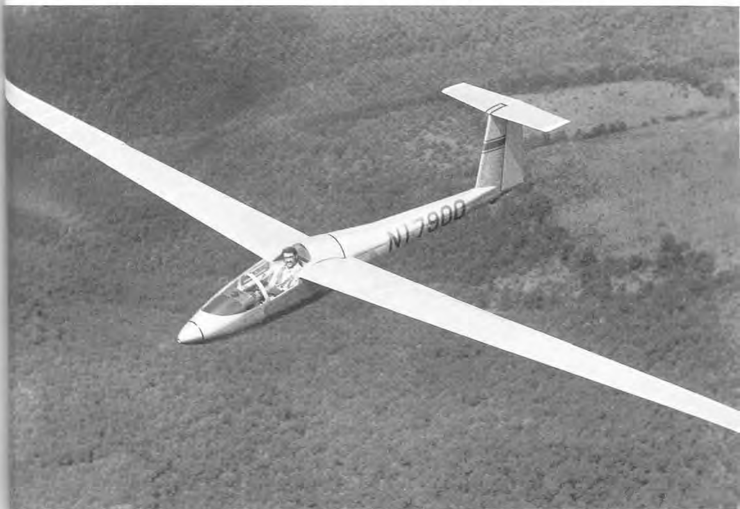
Les Schweizer flew the SGS 1-35 in natural aluminium finish. The two-piece cockpit canopy was peculiar to the prototype.
