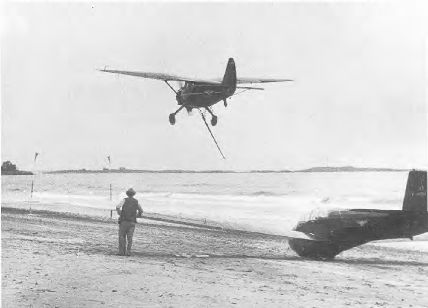
An All American Airlines Stinson tug picks up the A.A.A. lobster-carrying TG-3A from the Massachusetts beach. The long 'fishing rod' on the tug picked up the line suspended between the two poles, paying out line at first to avoid too great a jerk, and the glider took off smoothly and safely.
