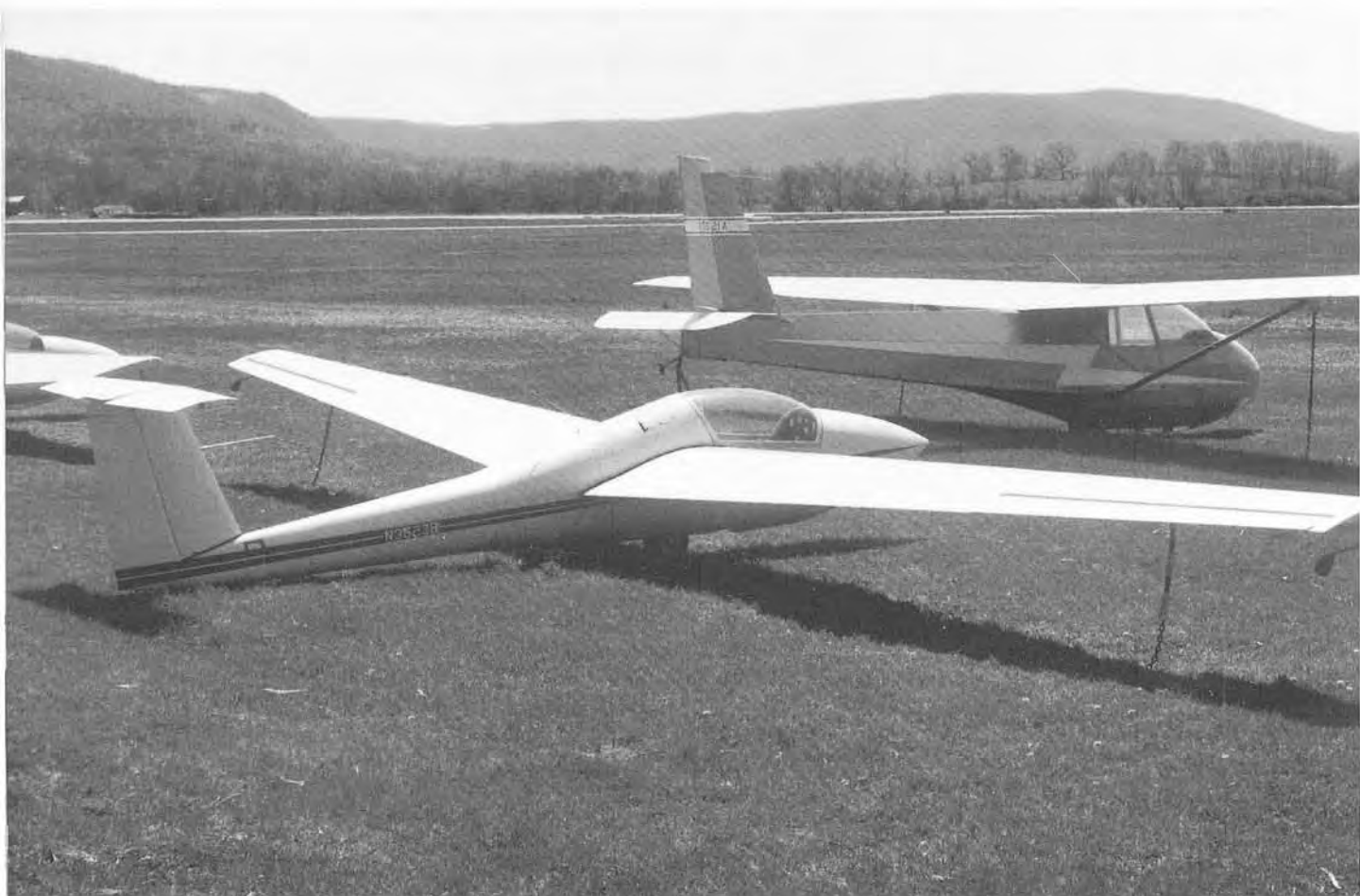
ABOVE: An SGS 1-36 at the Schweizer Soaring School at the start of the 1997 season. An orange and white 2-33 is seen behind. BELOW: Detail of the 1-36C version, with a forward-mounted landing wheel and no nose skid.
