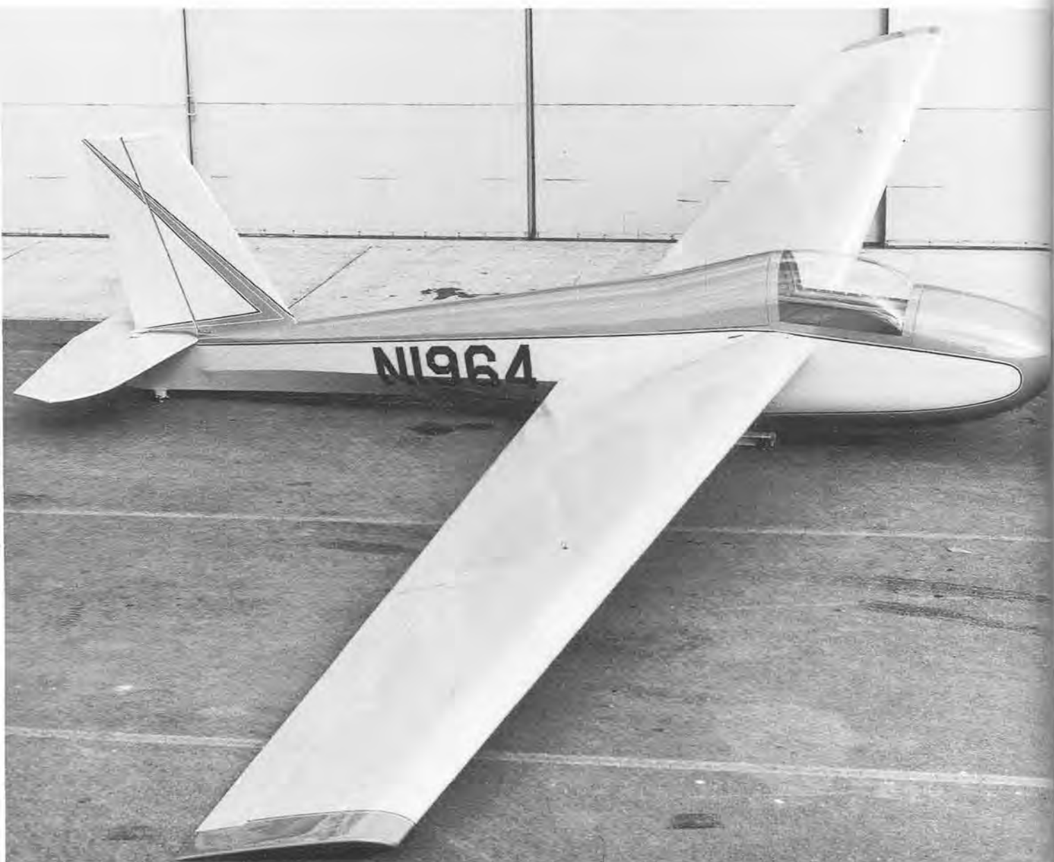
An SGS 1-26B with glassfibre nose skin, swept fin and special paint finish for an exhibition.
