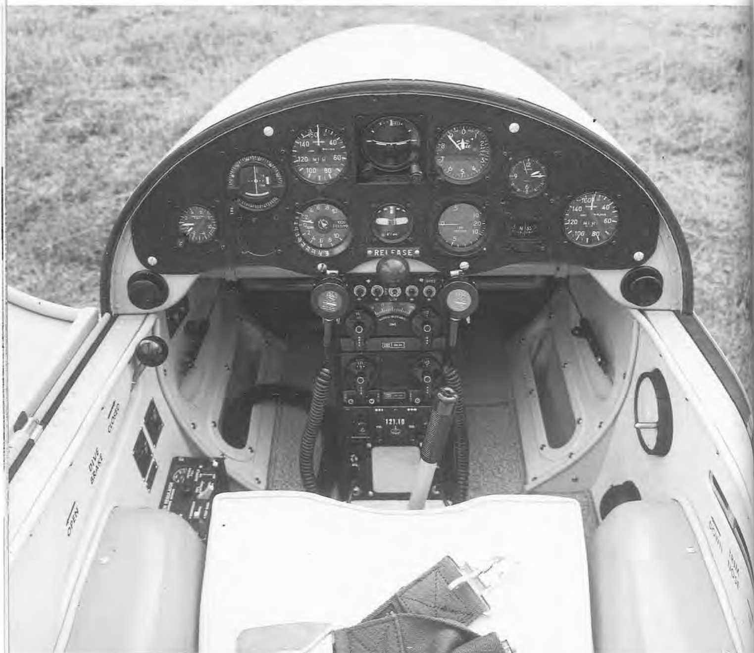
The SGS 2-32 Explorer sailplane for research into clear-air turbulence, showing the very complete instrumentation including 'Omni' navigational equipment.
