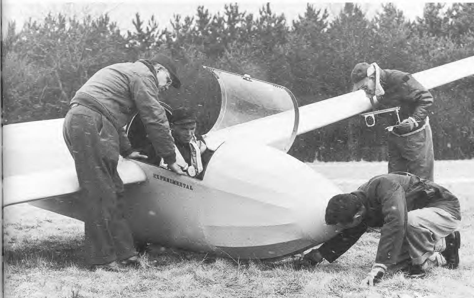
Paul Schweizer checks out Bob Smith for a first flight in the prototype SGS 1-26. Don Ryan adjusts the special calibration airspeed indicator, which is mounted on the wing, while a crewman hooks up the tow rope.
