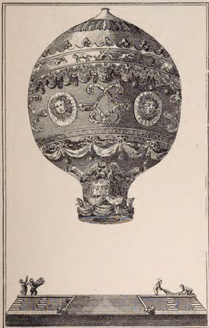
AEROSTATIC MACHINE, 70 FEET IN HEIGHT AND 46 FEET IN DIAMETER, WHICH ASCENDED FROM PARIS, WITH TWO MEN, TO A HEIGHT OF 324 FEET, ON THE 19TH OF OCTOBER, 1783.
