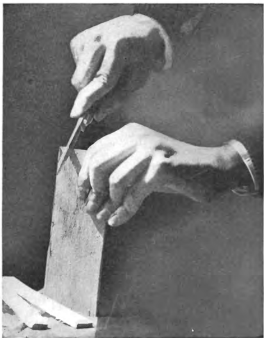
Splitting the Cigar Box Cover to Build the Propeller.
